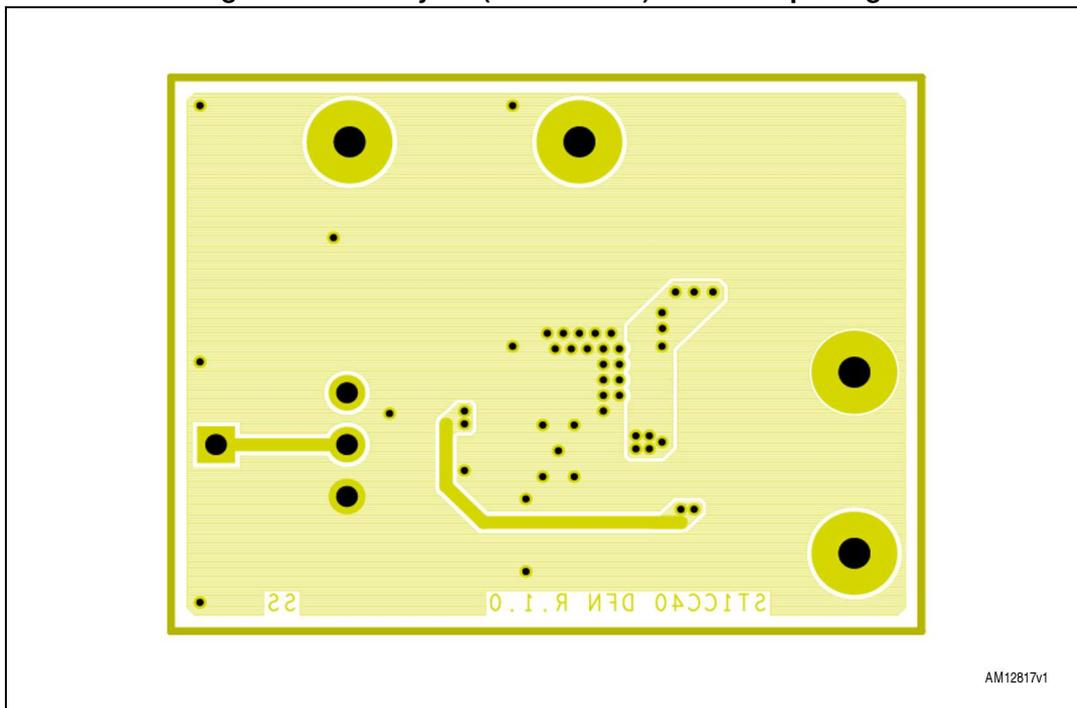
Figure 19. PCB layout (component side) SO8 package
