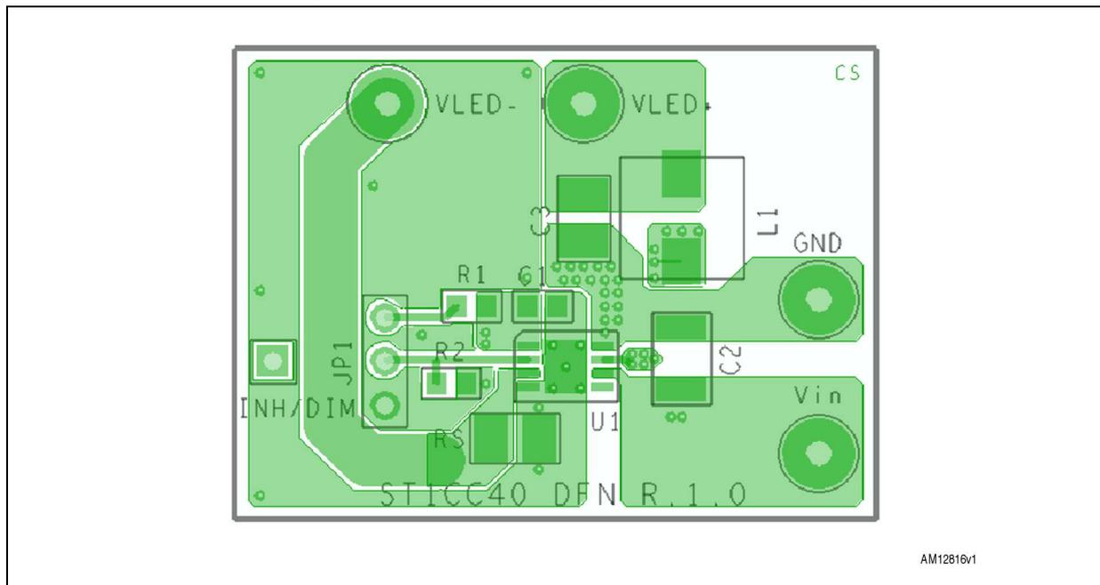
Figure 18. PCB layout (bottom side) VFQFPN8 package
