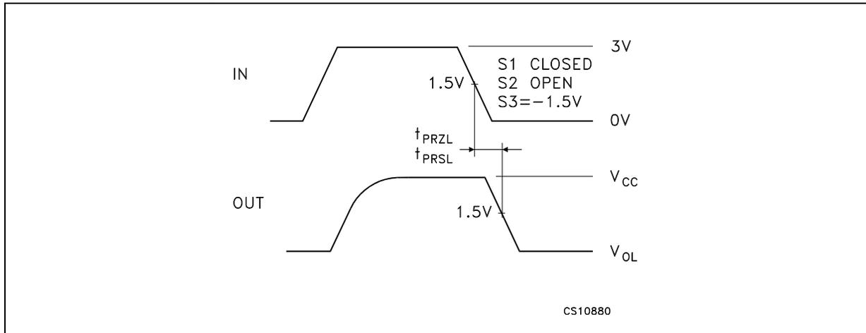
Figure 19. Receiver enable and disable times waveform
