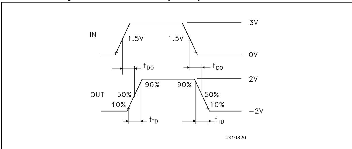
Figure 8. Drive enable and disable times test circuit
