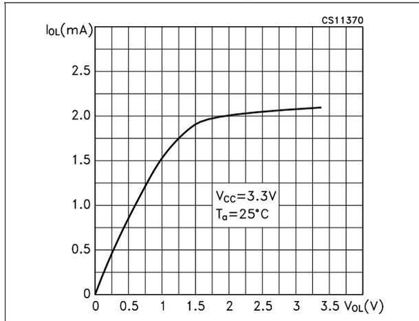
**Figure 22. Receiver output current vs output high voltage**
