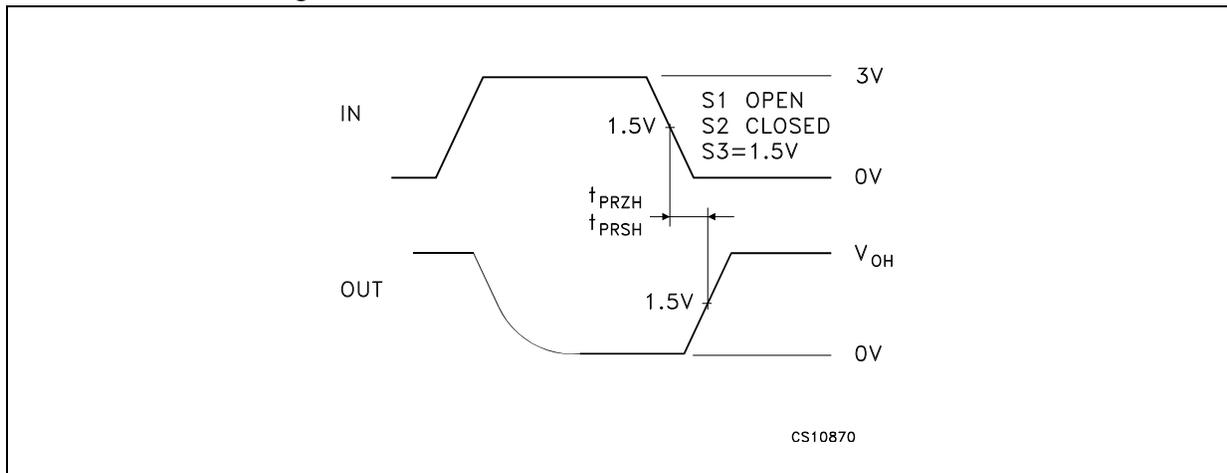
Figure 18. Receiver enable and disable times waveform
