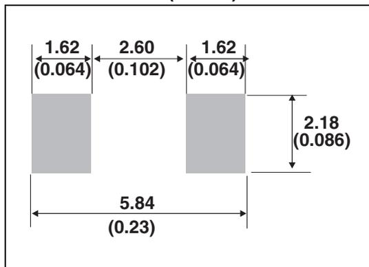
**Figure 8. Marking layout**
