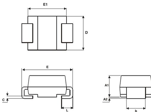
**Figure 20. Footprint dimensions in mm (inches)**
