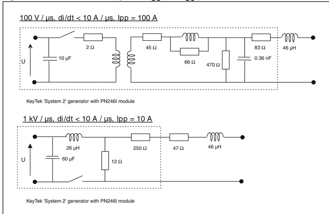
Figure 17. Test circuit 2 for  $I_{BO}$  and  $V_{BO}$  parameters
