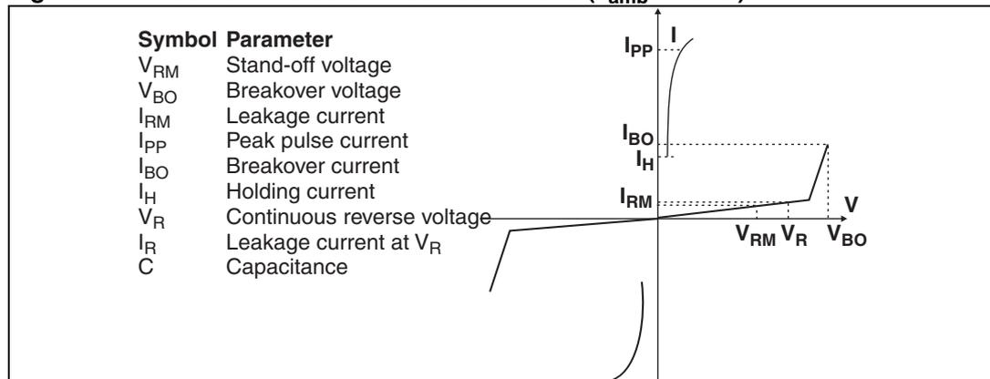
**Table 4. Electrical characteristics - values ( $T_{amb} = 25\text{ °C}$ )**
