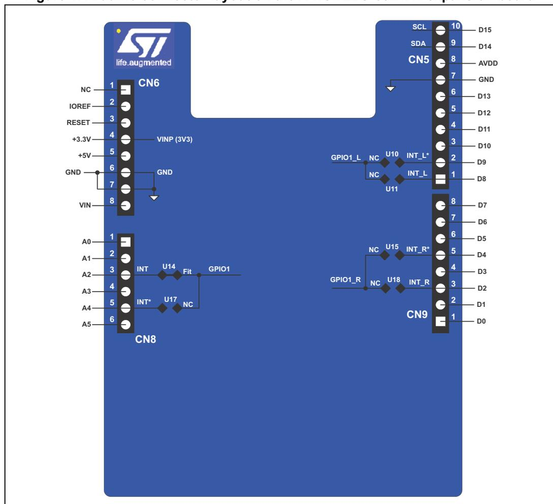
Table 1. Left connector of the Arduino on the NUCLEO-F401RE board
