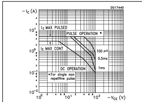
**Figure 3. Derating curve**
