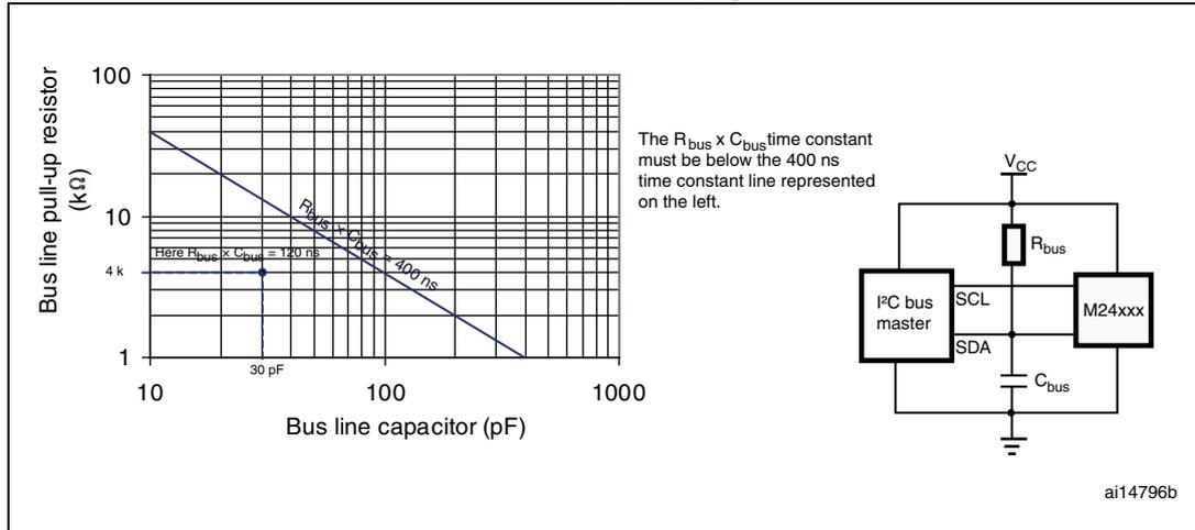
Figure 11. Maximum  $R_{bus}$  value versus bus parasitic capacitance ( $C_{bus}$ ) for an I<sup>2</sup>C bus at maximum frequency  $f_C = 1$  MHz
