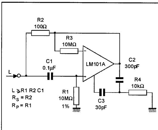
**FAST AMPLIFIER WITH HIGH INPUT IMPEDANCE**
