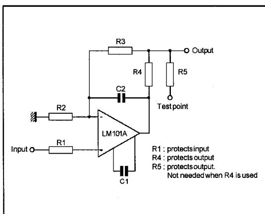
**COMPENSATING FOR STRAY INPUT CAPACITANCES OR LARGE FEEDBACK RESISTOR**
