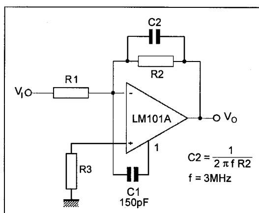
**PROTECTING AGAINST GROSS FAULT CONDITIONS**
