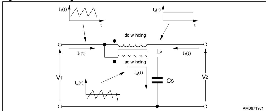
This application note, after reviewing the theoretical base, considers the realization of zero-ripple inductor current to minimize the input ripple in a TM PFC pre-regulator. In these systems, the large input ripple is one of the major limitations to its use at higher power levels.
