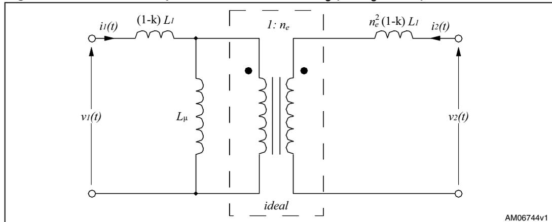
Another interesting and quite frequently used choice is  $a = 1$ . This results in a very simple model, illustrated in [Figure 27](#), useful for analyzing loosely coupled inductors, where  $L_1 - M$  and  $L_2 - M$  are both positive, which happens if:
