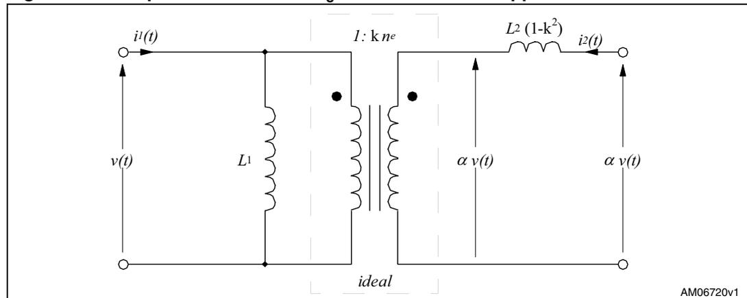
[Figure 4](#) shows that, in order for the secondary ripple current (i.e.  $di_2(t)/dt$ ) to be zero, the voltage across the inductance  $L_2 (1-k^2)$  must be zero, that is, the voltage on either side of it must be the same. Thereby:
