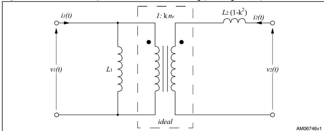
Other possible choices of  $a$  are  $a = M/L_1 = k n_e$ , which nulls  $L_a$  and puts all the elements related (logically, not physically) to the leakage flux on the secondary side (see [Figure 28](#)) and  $a = L_2/M = n_e/k$ , which nulls  $L_b$  and puts all the elements related to the leakage flux on the primary side (see [Figure 29](#)).
