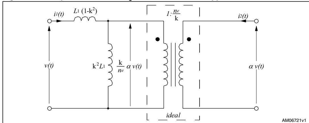
Similarly, considering the model of [Figure 5](#), again excited by proportional voltages  $v(t)$  and  $\alpha v(t)$ , it is equally apparent that, in order for the primary ripple current to be zero the voltage across the inductance  $L_1(1-k^2)$  must be zero, that is, the voltage on either side of it must be the same:
