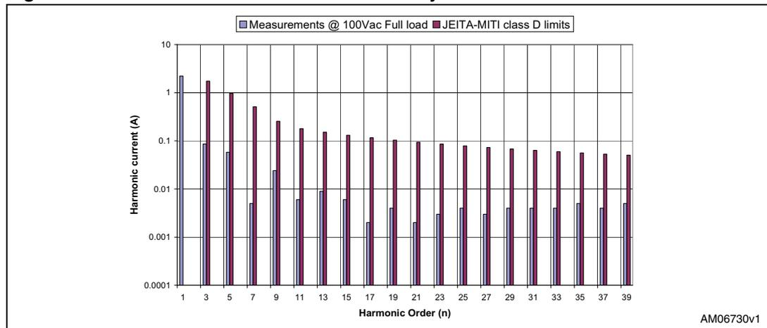
**Figure 15. Harmonic emissions and conformity to EN61000-3-2 standards**
