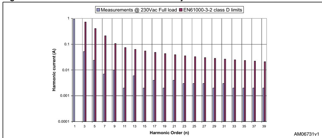
Figure 16. 200W PFC pre-regulator with ripple-free input current: typical performance
