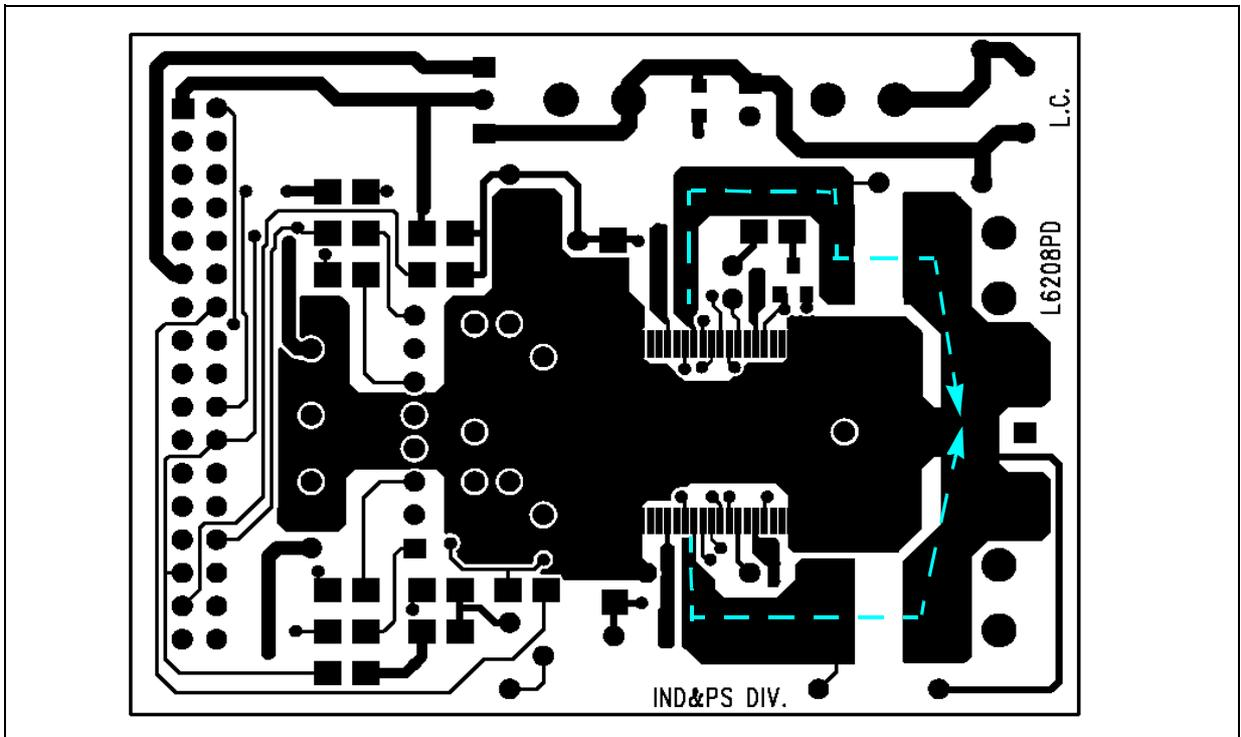
Figure 46. EVAL6208PD Bottom Layer Layout.
