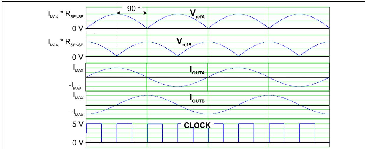
Especially at high rotation speeds, slow decay mode can be inadequate since it does not allow the motor current to decay fast enough, following the decreasing slope of the desired sine wave. In this case it's possible to apply the fast decay mode just during the negative slope of the current (see Figure 32). The disadvantage is an increased current ripple in the other winding (where the current is increasing and fast decay is not needed).
