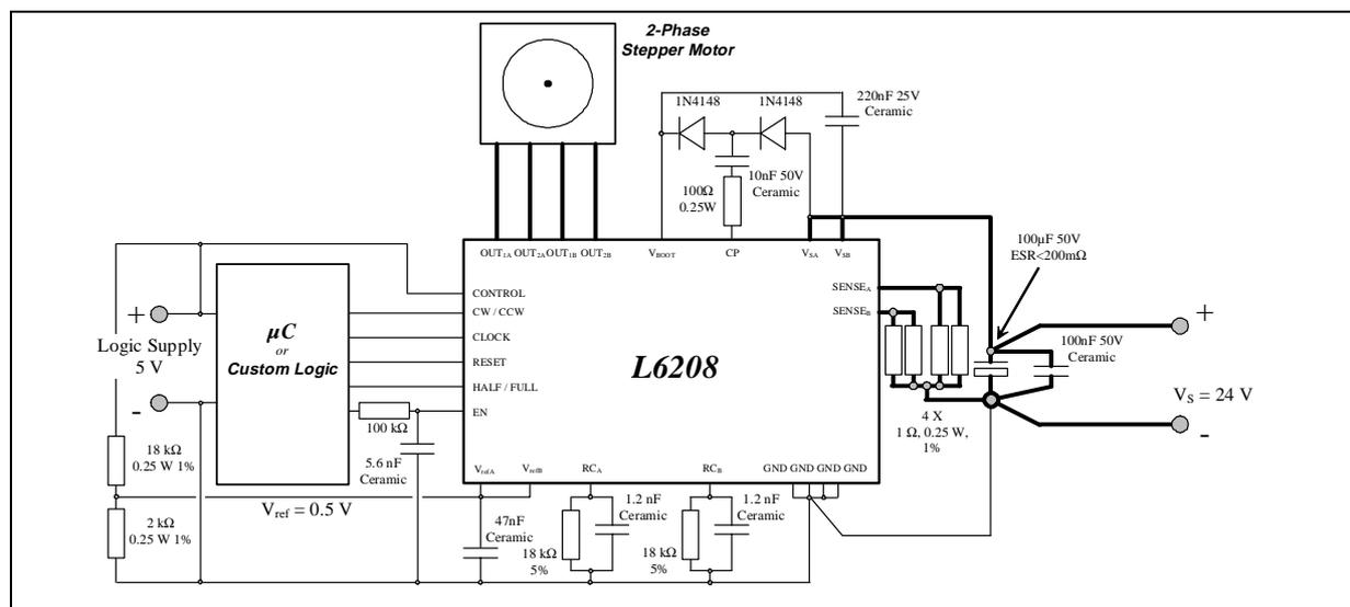
With Wave Drive selected, referring to Figure 24, Figure 25, Figure 26, the dissipating power is about 1.36 W. If the ambient temperature is lower than 50 $^\circ\text{C}$ , with 4cm $^2$  of copper area on the PCB and a SO24 package, the estimated junction temperature is about 123 $^\circ\text{C}$ . Using more copper area or a PowerDIP package will reduce the junction temperature.
