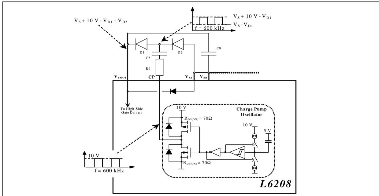
When the oscillator output is at ground,  $C_5$  is charged by  $V_S$  through  $D_2$ . When it rises to 10V,  $D_2$  is reverse biased and the charge flows from  $C_5$  to  $C_8$  through  $D_1$ , so the  $V_{BOOT}$  pin, after a few cycles, reaches the maximum voltage of  $V_S + 10V - V_{D1} - V_{D2}$ , which supplies the high-side gate drivers.
