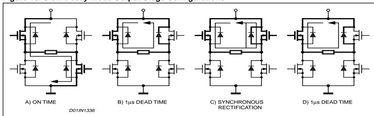
In some conditions (short off-time, very low regulated current, high motor winding L / R) the system may need an on-time shorter than 1.5µs. In these cases the PWM current controller can lose the regulation.
