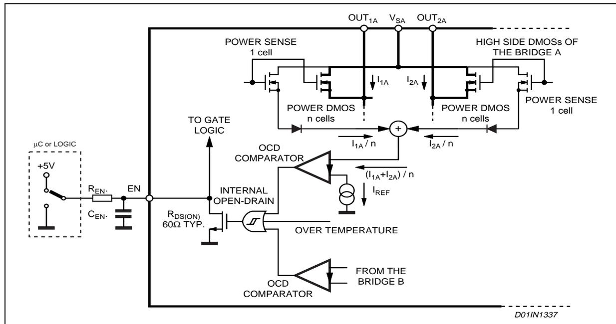
This sensed current is compared to an internally generated reference to detect an over current condition. An internal open drain mosfet turns on when the sum of the currents in the bridges 1A and 2A or 1B and 2B reaches the threshold (5.6A typical value); the open drain is internally connected to the EN pin. To ensure an over current protection, connect this pin to an external RC network (see Figure 18).
