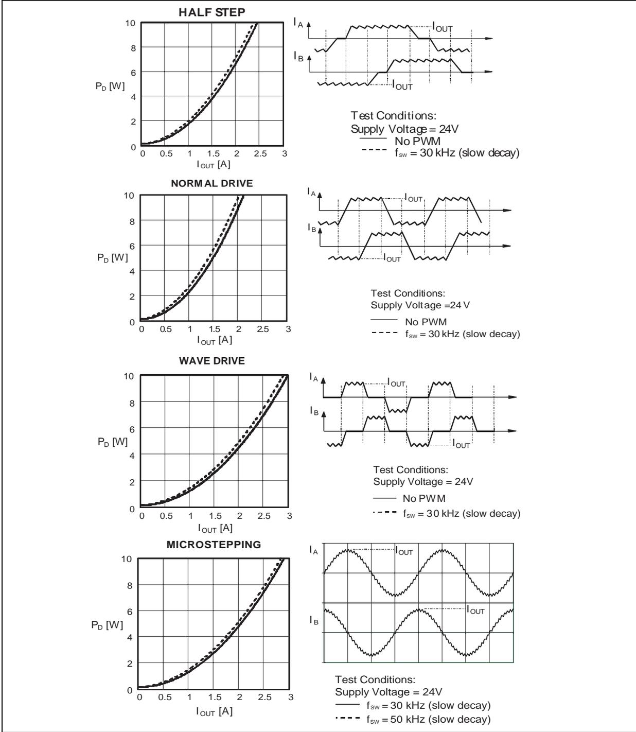
**2.13.1 Maximum output current vs. selectable devices**
