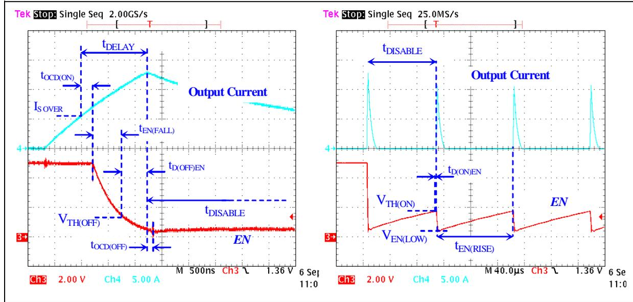
The maximum value reached by the current depends on its slew-rate, so on the short circuit nature and supply voltage, and on the total intervention delay ( $t_{DELAY}$ ). It can be noticed that after the first current peak, the maximum value reached by the output current becomes lower, because the capacitor on  $EN$  pin is discharged starting from a lower voltage, resulting in a shorter  $t_{DELAY}$ .
