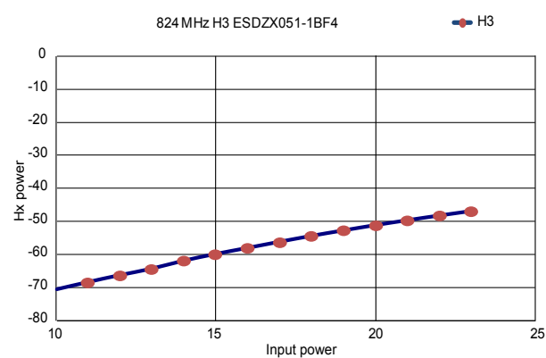
Figure 11. Harmonic measurement at 824 MHz : H3
