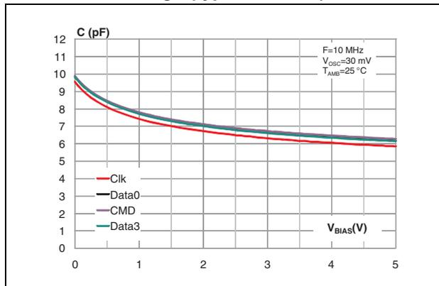
**Figure 6. Line capacitance versus frequency (typical values)**
