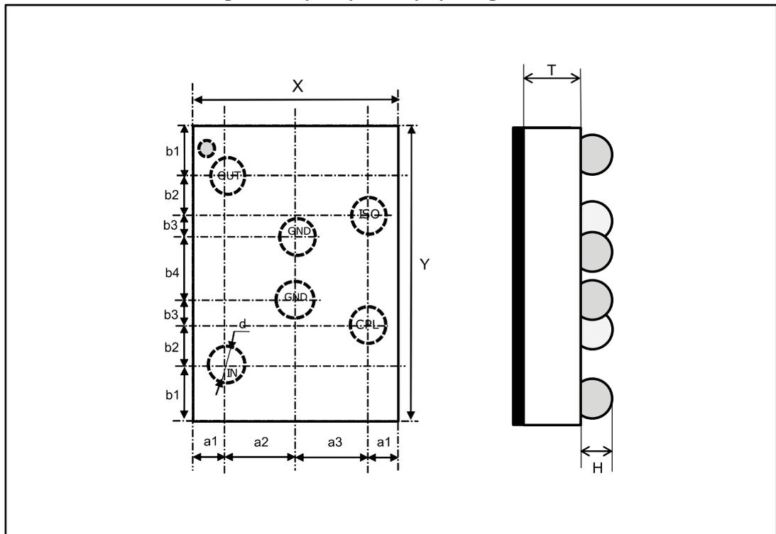
Table 4: Flip-Chip 6 bumps package mechanical data
