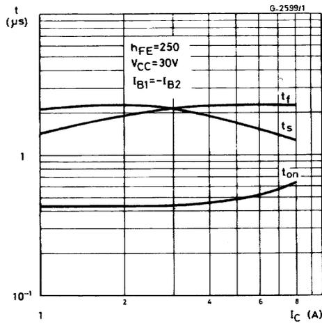
Saturated Switching Characteristics (PNP types)
