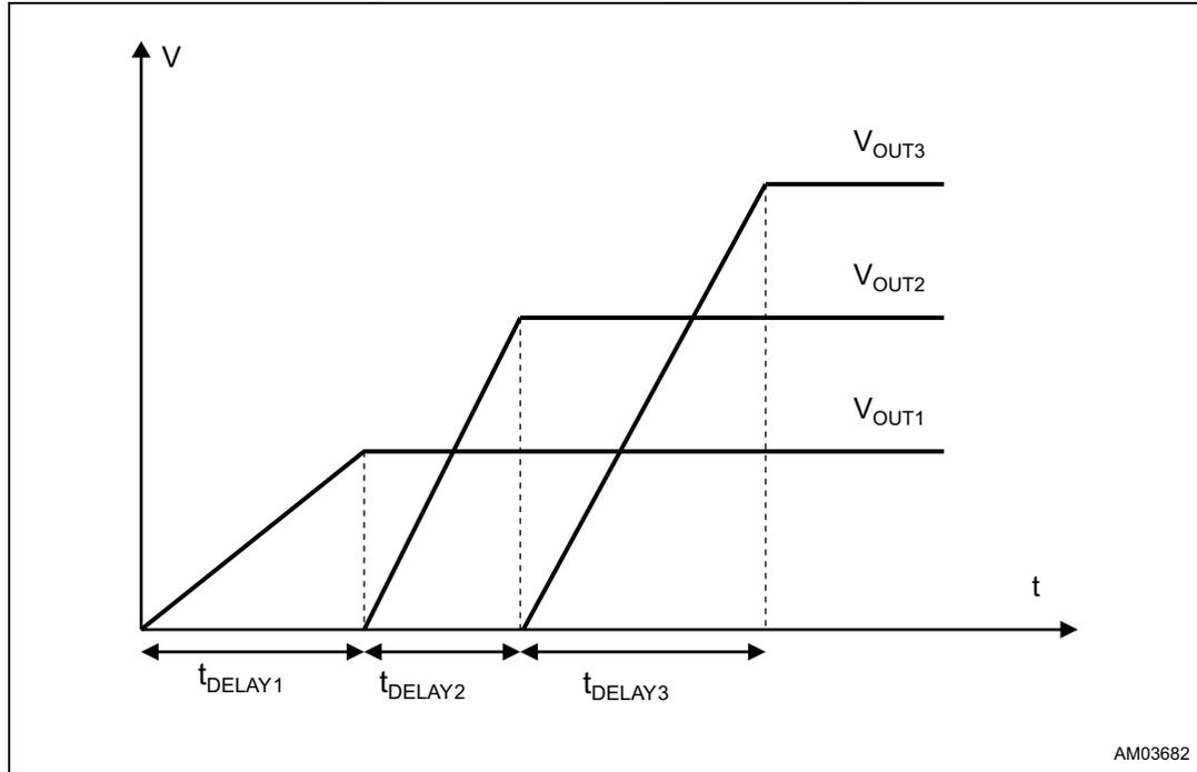
High flexibility is achieved thanks to the programmable RST thresholds (see [Table 7 on page 12](#), [Table 8](#) and [Table 9 on page 13](#)) and programmable delay time. To minimize the component count the DELAY pin capacitor can be also omitted so the pin works as a normal Power Good.
