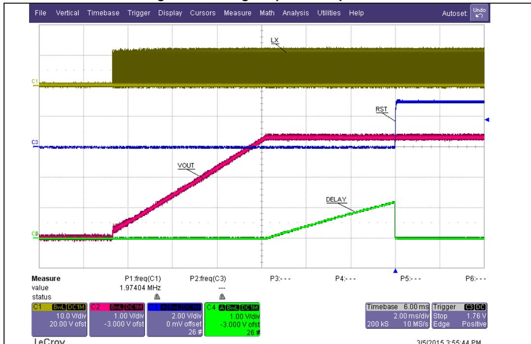
The comparator monitoring the FB voltage has four different programmable thresholds (80%, 87%, 93%, 96% nominal output voltage) for high flexibility (see [Section 7.3: MLF pin](#), [Table 7 on page 12](#), [Table 8](#), and [Table 9 on page 13](#)).
