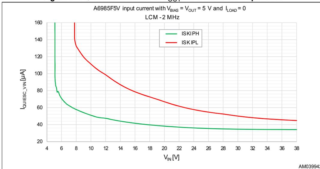
When  $V_{IN}$  approaches  $V_{OUT}$  (see zoomed [Figure 27](#) for the A6985F3V3 and [Figure 28](#) for the A6985F5V), the device increases the switching activity towards continuous conduction mode operation for the internal slope contribution effect on the programmed skip current threshold. As a consequence the quiescent current increases.
