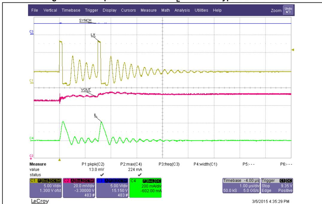
The LCM operation satisfies the requirements of the unswitched car body applications (KL30). These applications are directly connected to the battery and are operating when the engine is disabled. The typical load when the car is parked is represented by a CAN transceiver and a microcontroller in sleep mode (total load is around 20 - 30  $\mu\text{A}$ ). As soon as the transceiver recognizes a valid word in the bus, it awakes the  $\mu\text{C}$  and the rest of the application.
