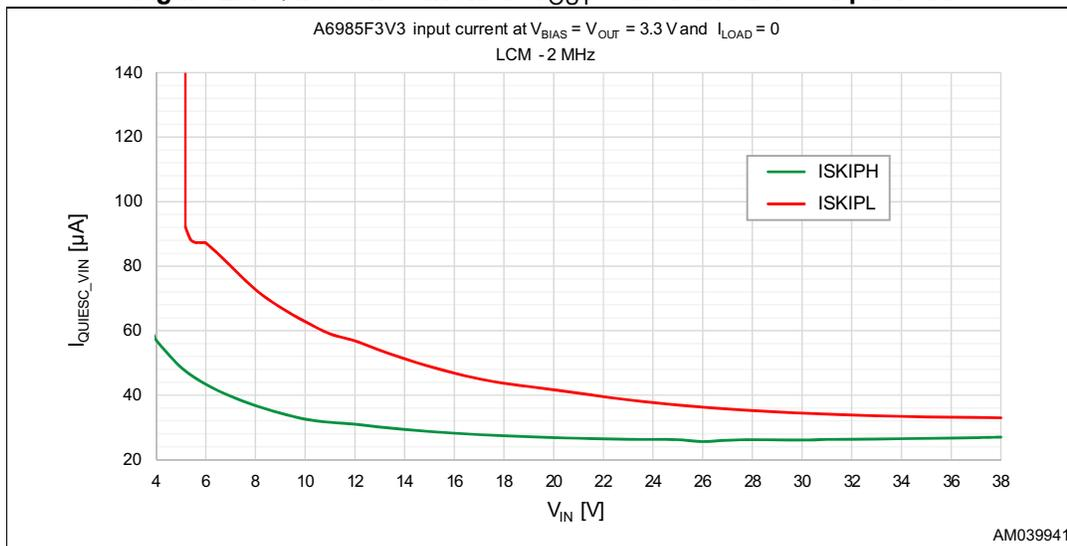
When  $V_{IN}$  is adequately higher than  $V_{OUT}$  (see [Figure 25](#) and [Figure 26](#)), the device works in the bursts mode operation, minimizing the power consumption (see [Section 5.8.2: Low consumption mode \(LCM\)](#)).
