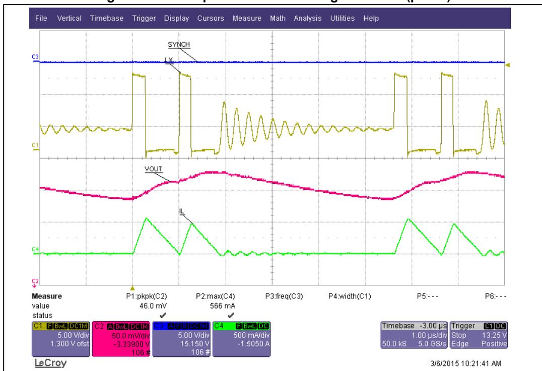
Figure 23. LCM operation over loading condition (part 2)
