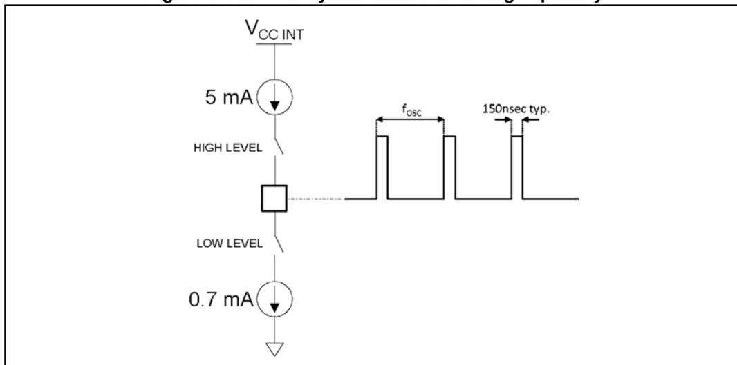
In order to safely guarantee that each regulator recognizes itself in SLAVE mode during the normal operation, the external master must drive the SYNCH pin with a clock signal frequency higher than the maximum oscillator spread (refer to [Table 6](#)) for at least 10 internal clock cycles.
