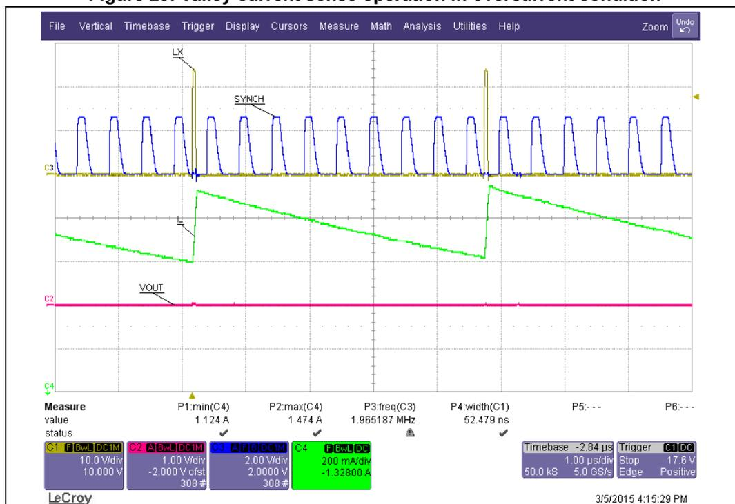
Figure 29 shows the switching frequency reduction during the valley current sense operation in case of extremely low duty cycle ( $V_{IN} = 38$  V,  $f_{SW} = 2$  MHz short-circuit condition).
