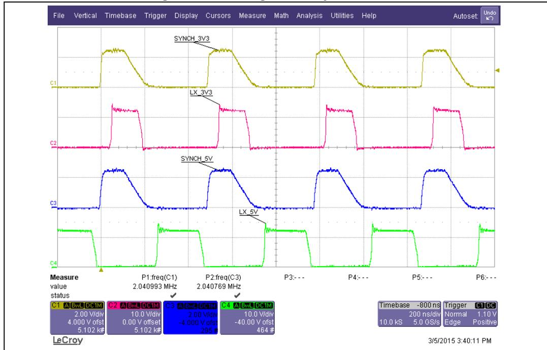
Multiple A6985F devices can be synchronized to an external frequency signal fed to the SYNCH pin. In this case the regulator set is phased to the reference and all the devices will work with 0° phase shift.
