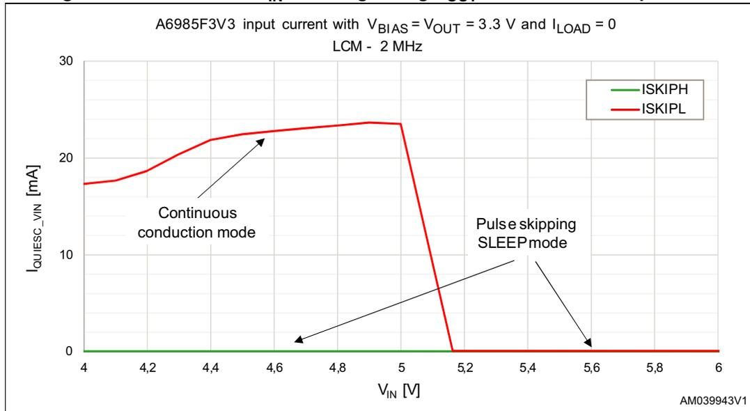
When  $V_{IN}$  is lower than  $V_{OUT}$  (see [Figure 28](#)), the device enters into the low dropout operation with the high-side always switched on. In this operating condition, all the internal circuit blocks are active and the quiescent current corresponds to what measured in the low noise mode operation (see  $I_{Q\ OP\ VIN}$  and  $I_{Q\ OP\ VBIAS}$  in [Table 5: Electrical characteristics on page 9](#) given  $V_{FB} = GND$ ).
