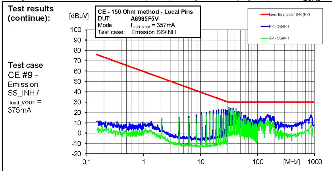
Figure 74. CE 150R at SS/INH test point (see Figure 66) at 10% I<sub>LOAD</sub>
