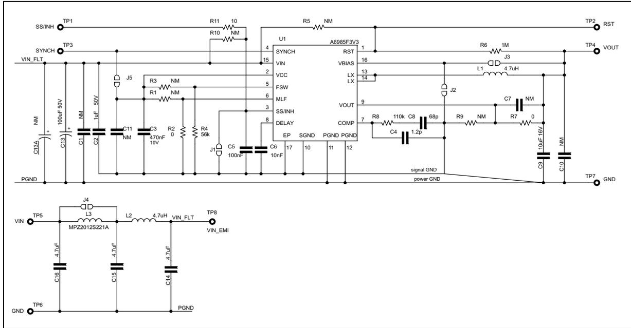
The additional input filter (C16, L3, C15, L2, C14) limits the conducted emission on the power supply (refer to [Figure 64 on page 72](#)).
