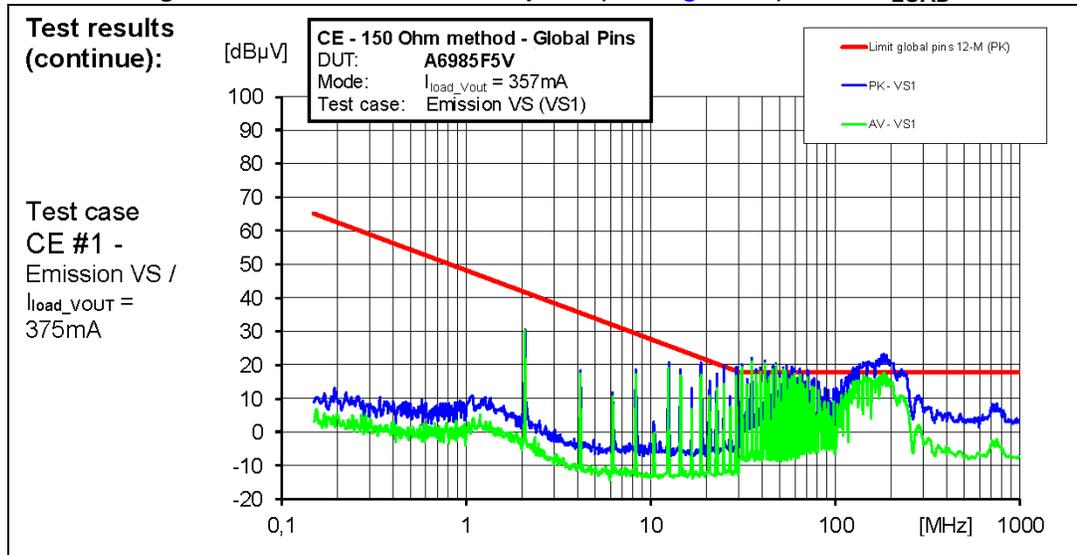
Figure 68. CE 150R at VS1 test point (see Figure 66) at 10% I<sub>LOAD</sub>
