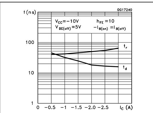
Figure 8. Resistive load switching times
