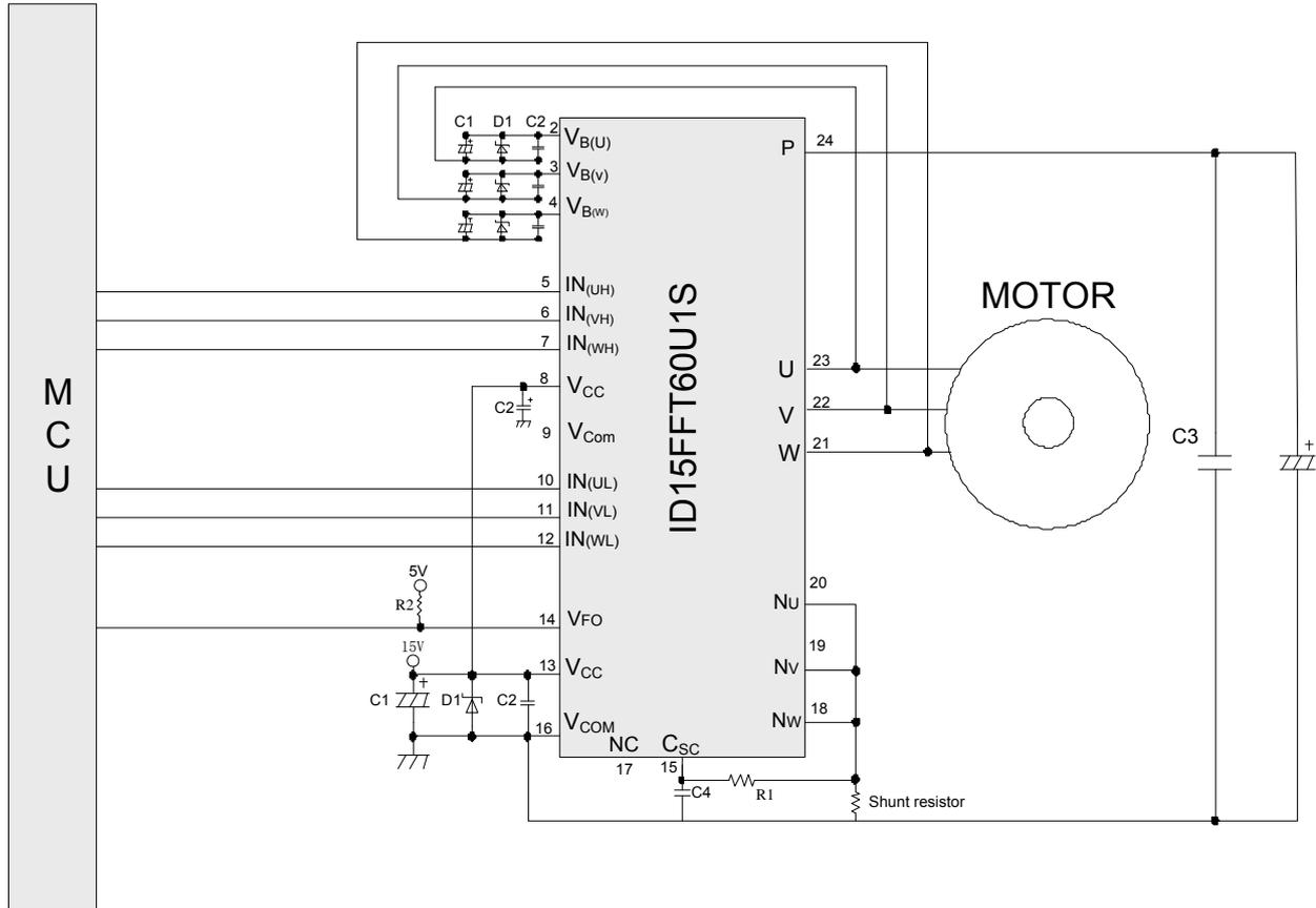
Figure 12. Typical Application Circuit Interface Example without Photo-Coupler
