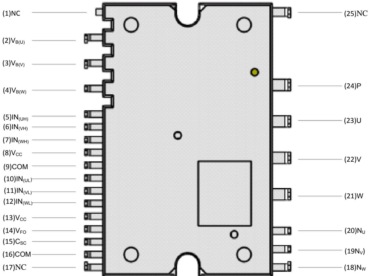
Figure 2. Pin Configuration
