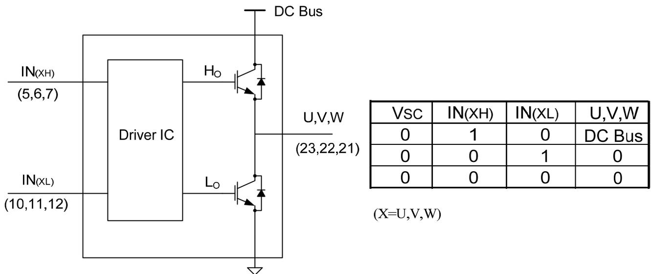
Figure 9. Input/Output Signal Circuit
