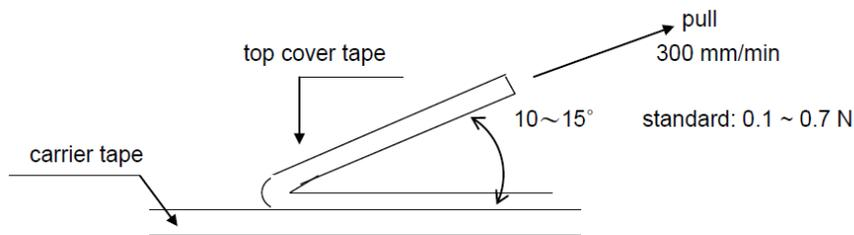
Peel-off force of paper and blister tape is in accordance with "JIS-C5202", that is, 0.1 to 0.7N at a peel-off speed of 300 mm/minute.
