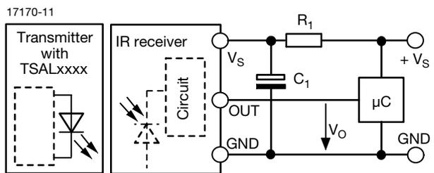
R<sub>1</sub> and C<sub>1</sub> recommended to reduce supply ripple for V<sub>S</sub> < 2.8 V
