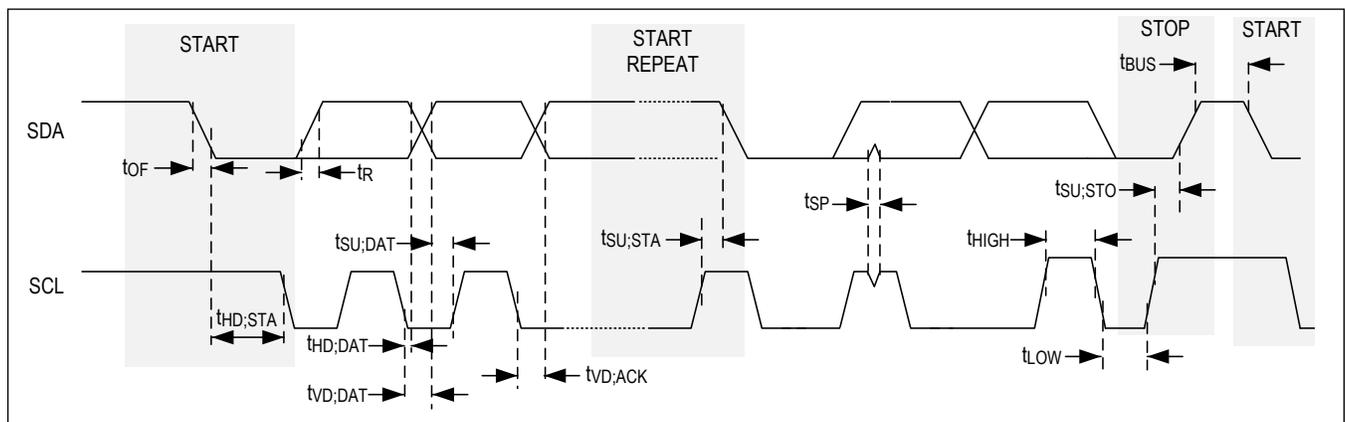
Figure 1. I<sup>2</sup>C Timing Diagram
