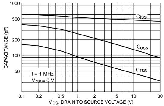
Figure 8. Capacitance Characteristics.
