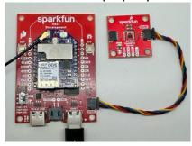
2. Confirm that the switch on the lower left side of the Development Board is in the down position for I2C. If this switch is set incorrectly the sensor will not be able to communicate, so it's very important!
