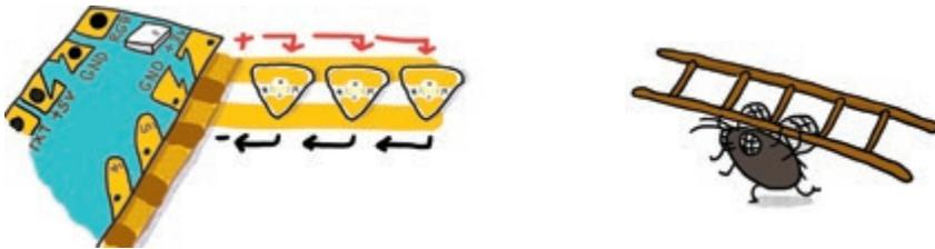
As the illustration above shows, all of the (+)'s go to the +3V pin, and all of the (-)'s connect to ground. This way the power source provides enough voltage ("height") for each LED. Since each LED needs at least 2.5V, connecting them in parallel to the +3V pin will turn all the LEDs on.
