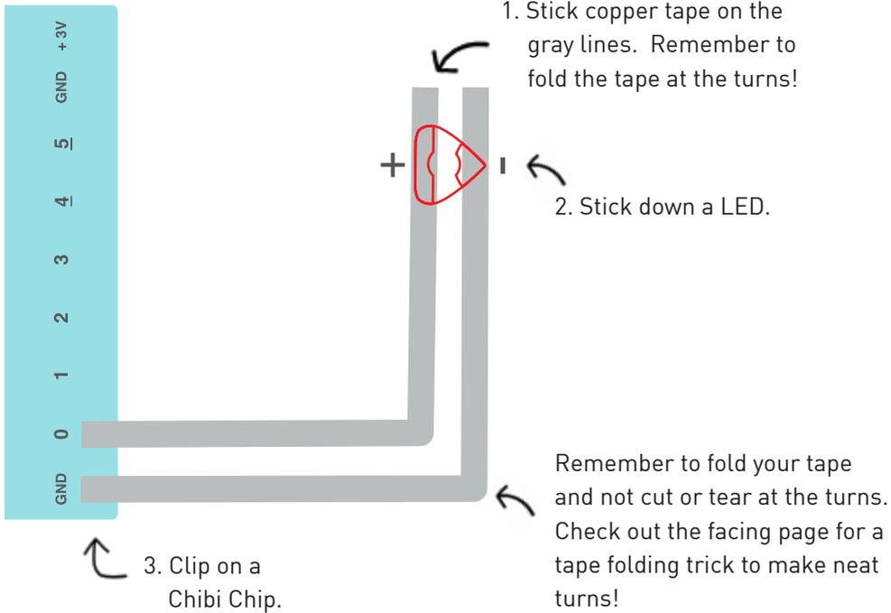
See how when you connect the LED circuit to pin 0, the LED also blinks just like the indicator light on the Chibi Chip? That's because the pin sends power to both the light on the Chip as well as to any LEDs in a circuit connected to that pin.
