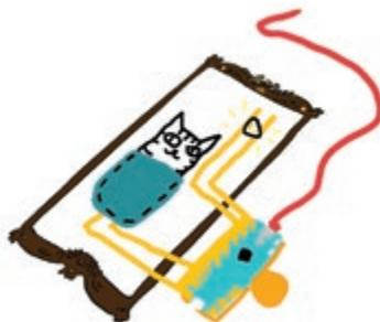
Here's what the finished pocket character switch looks like. When we put the cat in the pocket, it will close the circuit, turning the switch on. Make sure to push the cat all the way into the pocket for a secure connection.
