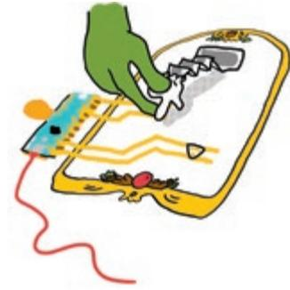
Here's what the finished pop-up switch looks like! Stretch the pointer finger so reaches the switch contacts, and then press to activate the switch. When we let go, the pointer springs back up!
