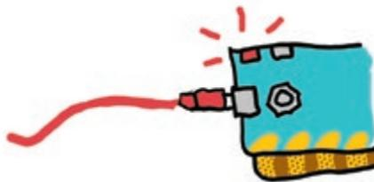
If this happens, unplug the Chibi Chip from the power source, find the connection causing the short circuit, and remove it. To learn more about short circuits, go to page **1-8**.
