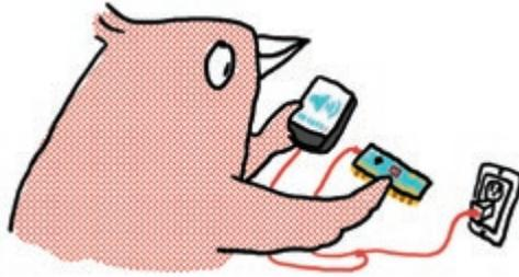
5. Press and hold the program button on the Chibi Chip until the PROG light stays red. This lets the Chibi Chip know to listen for new code. Let go of the button after the light turns red.
