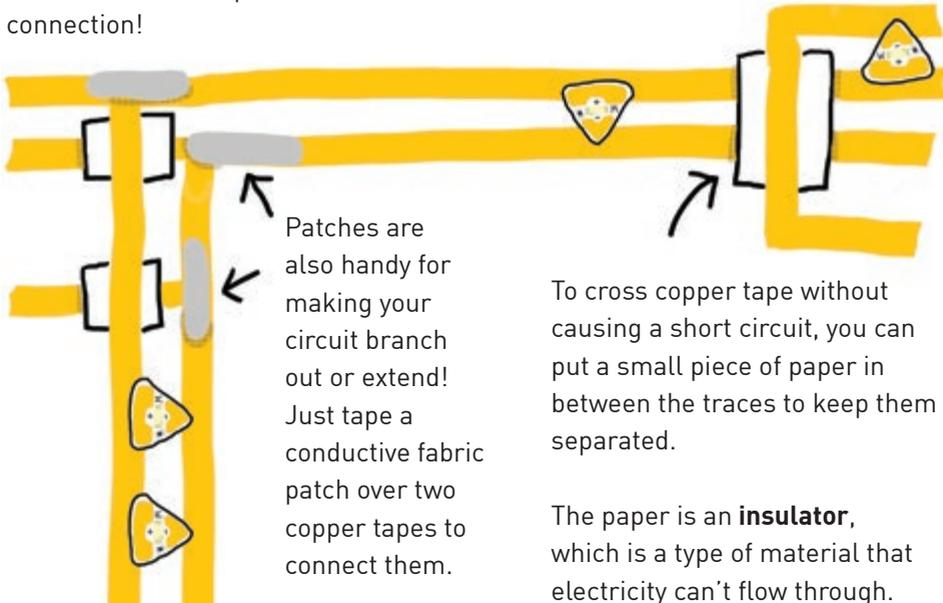
Patches are also handy for making your circuit branch out or extend! Just tape a conductive fabric patch over two copper tapes to connect them.
