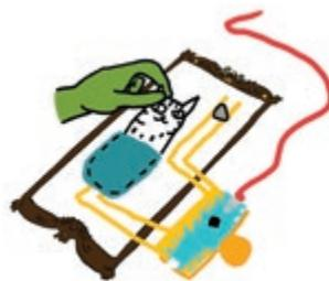
We can turn off the switch by pulling the cat out of the pocket, or by flipping the cat around so that the copper tape doesn't touch the circuit.
