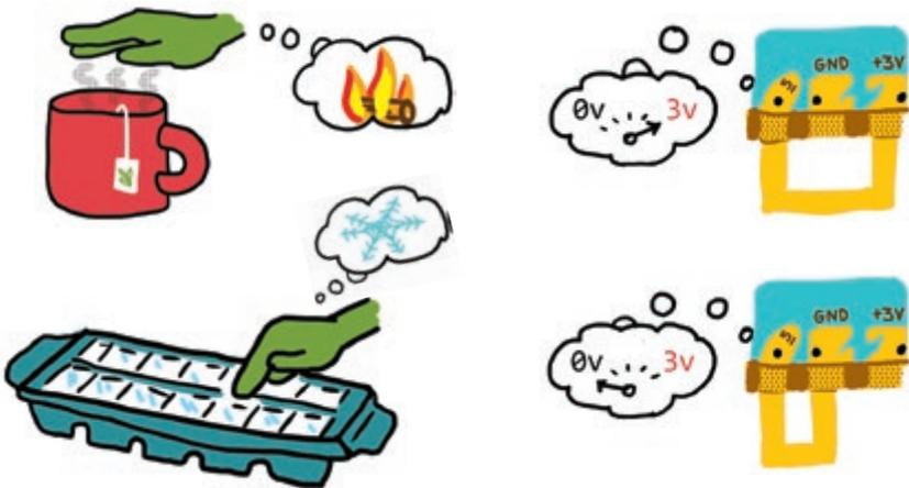
The code in the microcontroller processes the information from reading the input voltage to make choices and compute the proper output. We save the voltage reading in our `pressed` variable, process it through the `if()` statement, and then turn on or off the LED.
