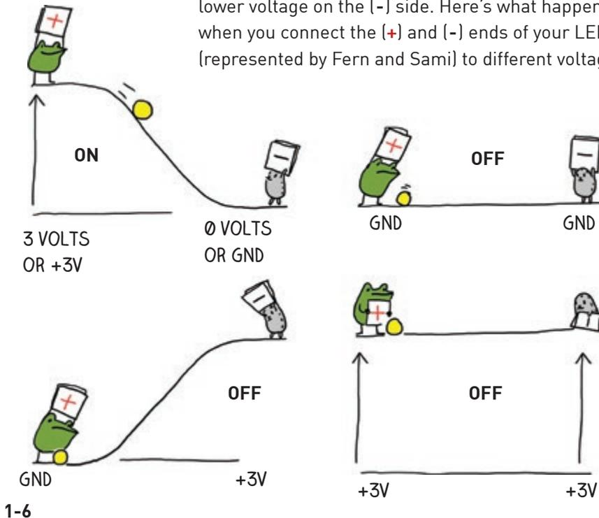
To summarize: when we connected the (+) side of the LED sticker to 3 volts and the (-) side to GND (or 0 volts), we provided enough voltage in the right direction for the LED to turn on!
