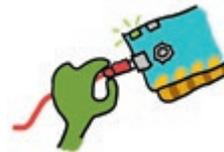
4. Align and clip the Chibi Chip to the page over this rectangle. Make sure the metal pads of the clip touch your circuit.
