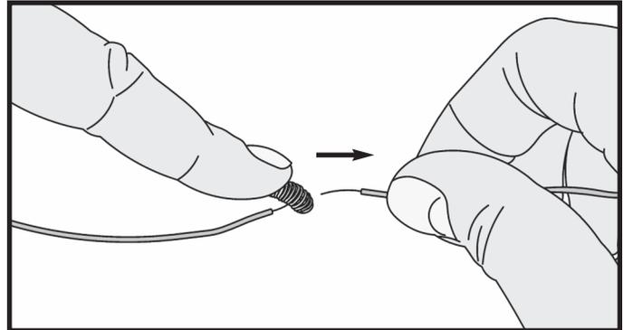
If the exposed metal ends of some of the wires break off due to great use, you should just simply remove 3/8" if the insulation from the wire of the broken end and then simply twist the strands together. To remove the installation you can use either a wire-stripper tool or a simple penknife. Be extremely careful when doing this because penknives are remarkably sharp.
