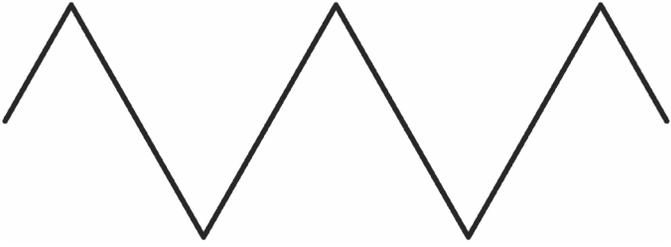
The shape of this wave results from the slow charging of the  $0.1\mu\text{F}$  capacitor through the control and the  $100\text{k}\Omega$  resistor, and the capacitor's discharge through the PNP and NPN transistors.
