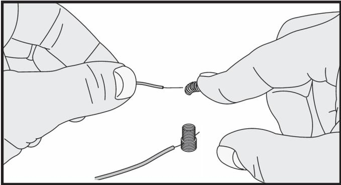
When you have to join two or three wires into a single spring terminal, be sure that the first wire does not come loose when you attach the second and third wires. The simplest way to do this is to place the spring onto the opposing side where you have connected the first wire.
