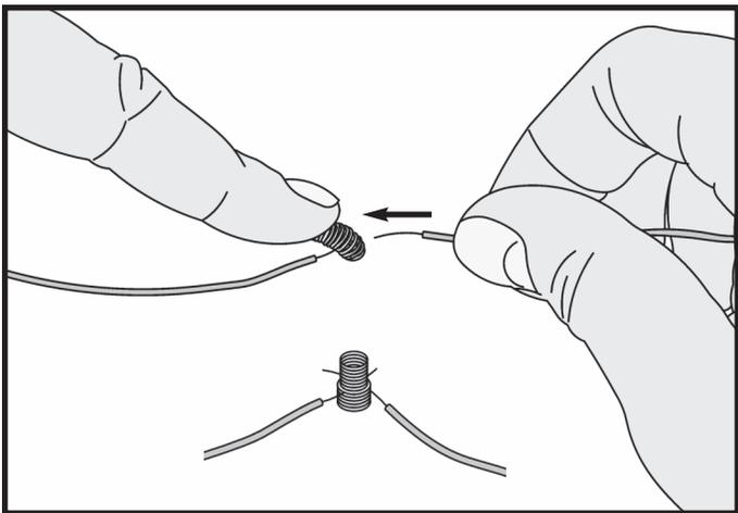
Only insert the exposed or shiny part of the wire into the spring terminal. The electrical connection will not be made if the plastic part of the wire is inserted into the terminal. Removing the wire from the spring terminals is simply just bending each terminal and then pulling the wires out of it.
