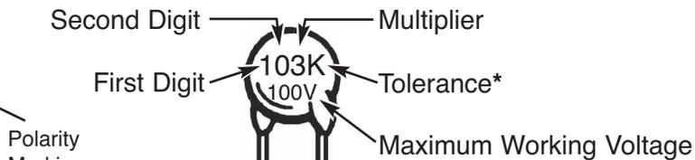
The value is  $10 \times 1,000 = 10,000\text{pF}$  or  $.01\mu\text{F}$  100V
