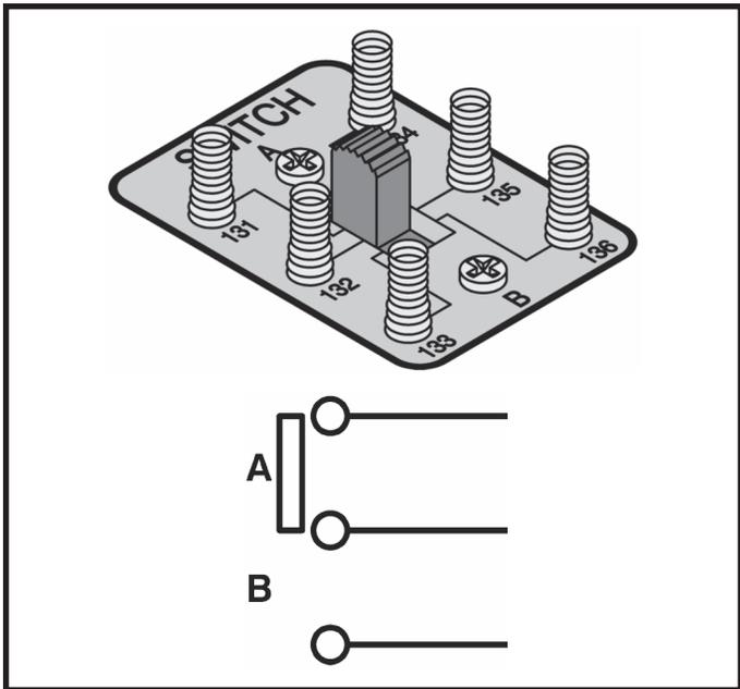
**Key:** The key is a simple switch—you press it and electricity is allowed to flow through the circuit. When you release it, the circuit is not complete because a break is caused in the circuit’s path. The key will be used in most circuits often times in signaling circuits (you can send Morse code this way as well as other things).
