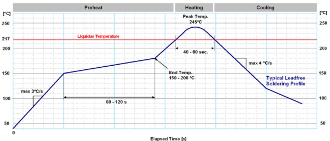
Figure 52: Soldering profile for professional grade ZED-F9P
