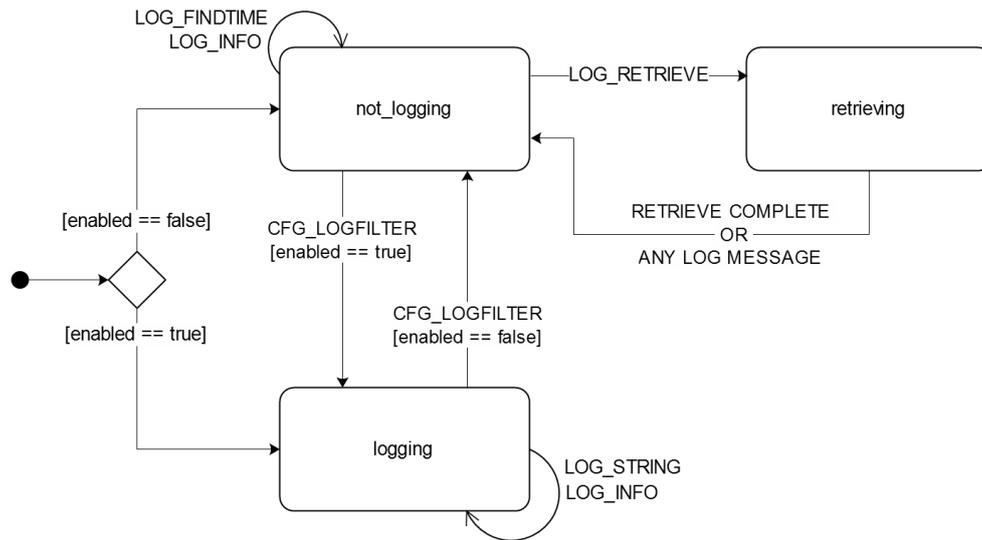
Figure 12: The states of the active logging subsystem
