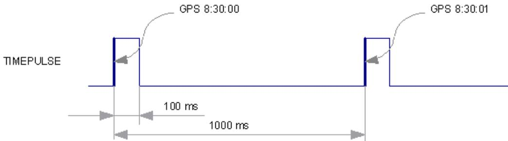
Figure 27: Time pulse signal with the example parameters
