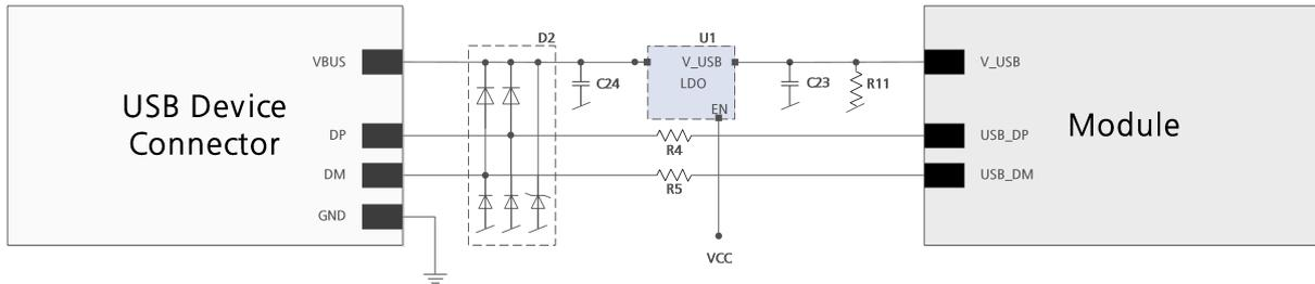
**Figure 23: ZED-F9P example circuit for USB interface**
