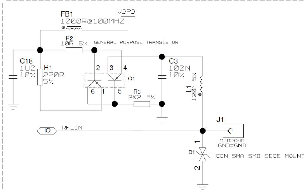
Figure 42: ZED-F9P reference design for antenna bias
