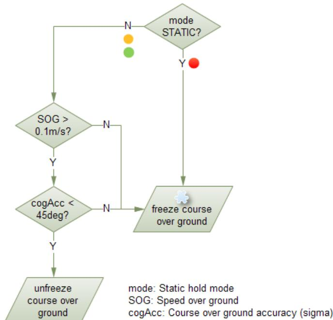
Figure 8: Flowchart of the course over ground freezing
