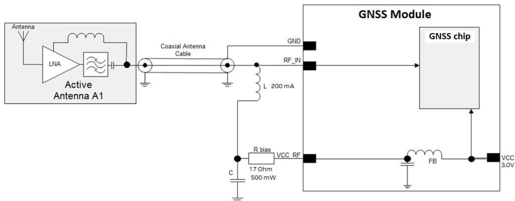
Figure 43: ZED-F9P VCC\_RF antenna bias
