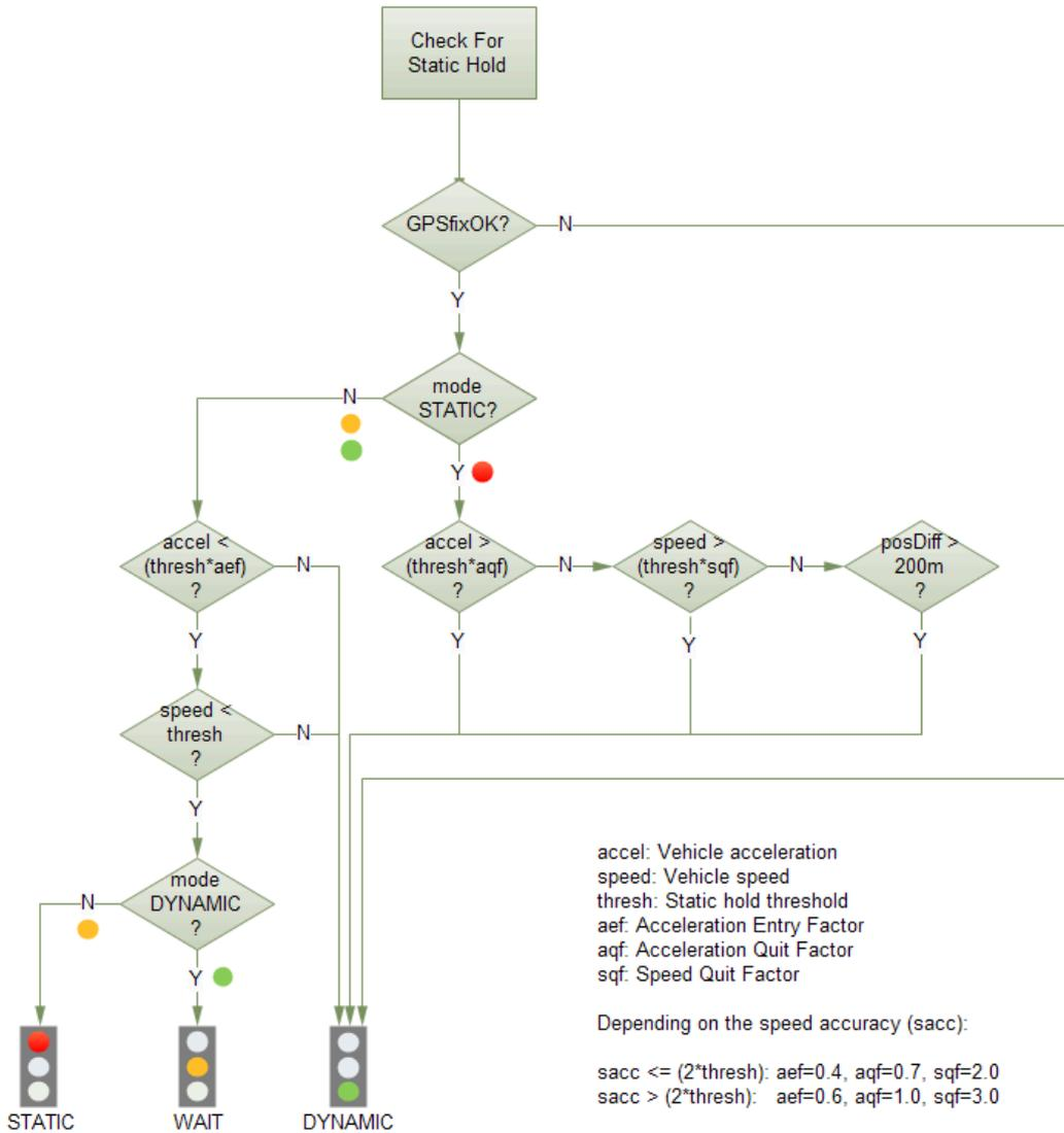
Figure 7: Flowchart of the static hold mode
