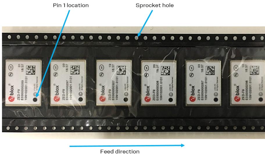
**Figure 53: Orientation of ZED-F9P on the tape**
