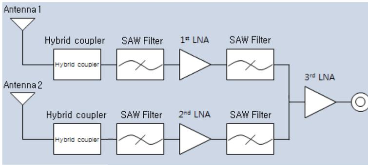
**Figure 40: u-blox low cost dual-band antenna internal structure**
