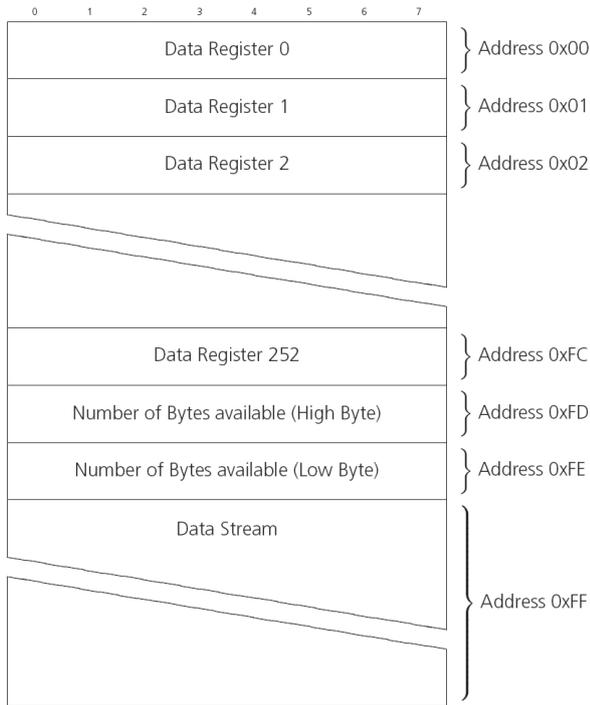
**Figure 18: I2C register layout**
