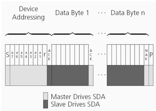
**Figure 20: I2C current address read access**
