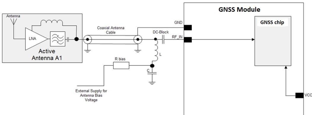
Figure 44: ZED-F9P external voltage antenna bias
