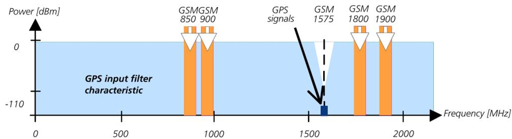
**Figure 15: Out-of-band interference signals**
