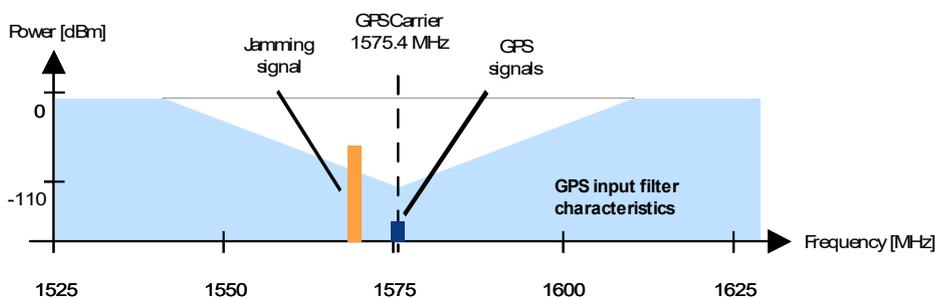
Figure 13: In-band interference signals
