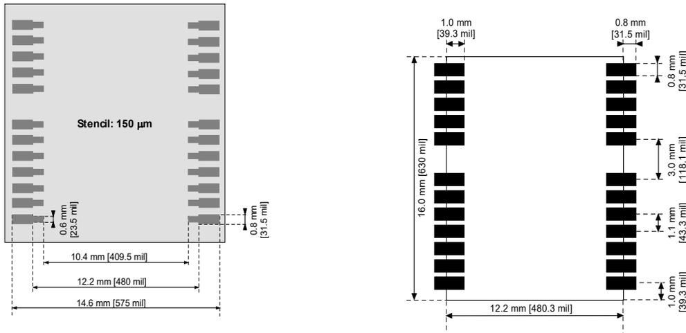
Figure 5: NEO-M8P paste mask / NEO-M8P footprint
