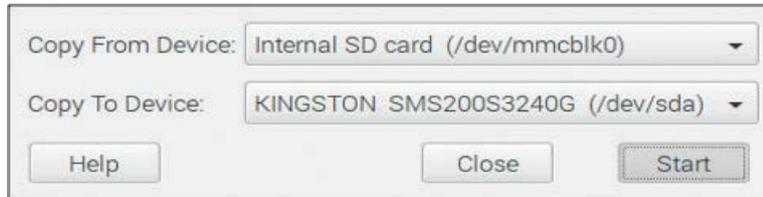
**Note:** If booting from SSD, ensure there are no other USB Flash Disks plugged into your Pi Desktop as this may result in an error of the Raspberry Pi not finding the correct boot device.
