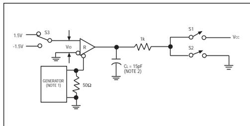
Figure 7. Receiver Enable and Disable Timing Circuit
