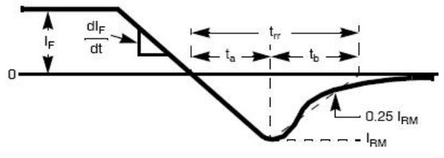
**Figure 11. Diode Reverse Recovery Waveform**
