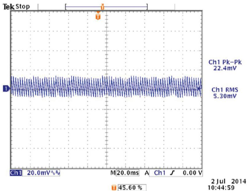
To verify that the output ripple and noise does not exceed the level specified in the product specification, measured using a scope probe socket with 0.1uF ceramic and a 10uF electrolytic capacitor connected in parallel across it, 20MHz BW.
