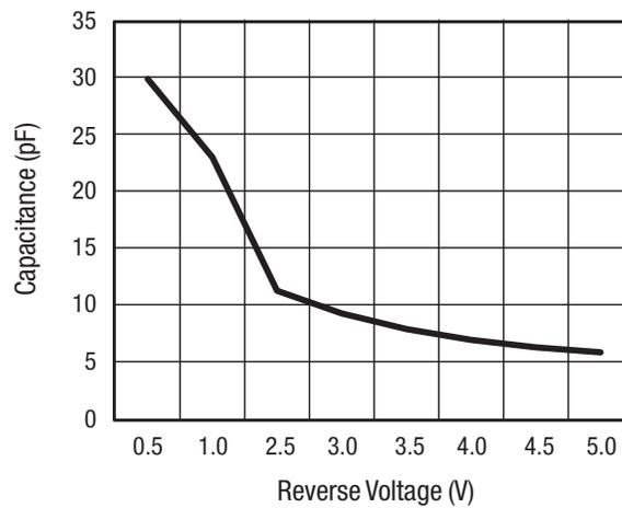
**Figure 1. Capacitance vs Reverse Voltage, Mean Test Data**
