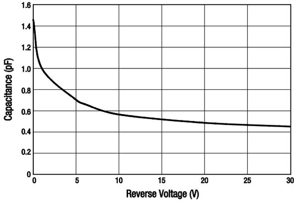
Figure 1. Capacitance vs Reverse Voltage @ 1 MHz
