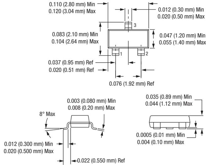
Dimensions are in inches (millimeters shown in parentheses)
