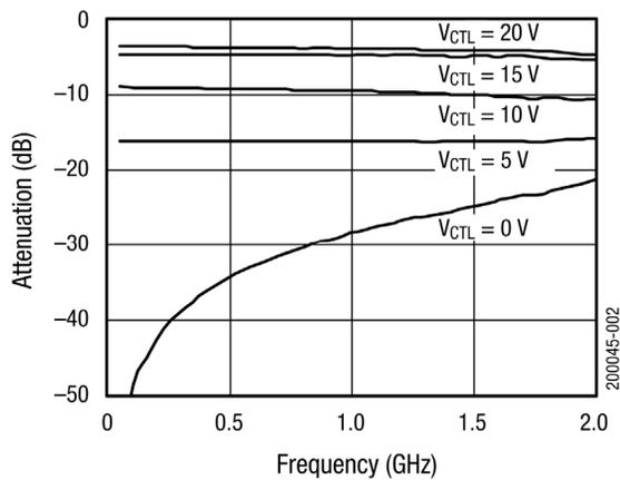
**Figure 2. SMP1307-027LF Attenuation vs Frequency vs Control Voltage**
