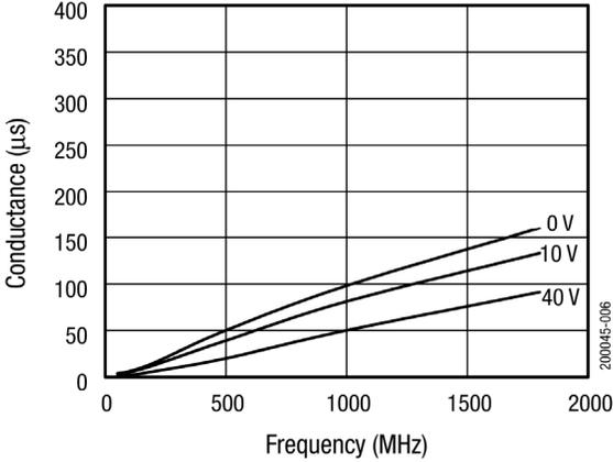
Figure 6. Conductance vs Frequency and Reverse Voltage
