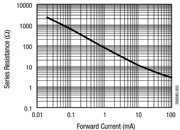
**Figure 3. Series Resistance vs Current @ 100 MHz**
