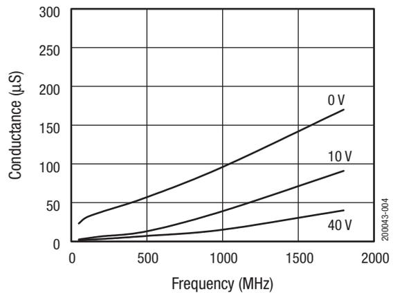
**Figure 4. Conductance vs Frequency and Reverse Voltage**
