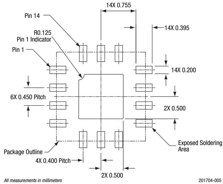
**Figure 5. SKY13415-485LF PCB Layout Footprint (Top View)**
