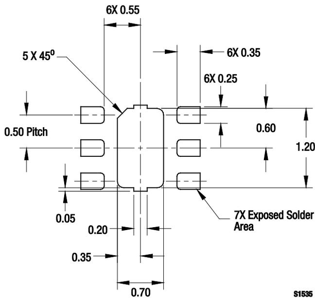
Figure 9. SKY13381-374LF PCB Layout Footprint (Top View)
