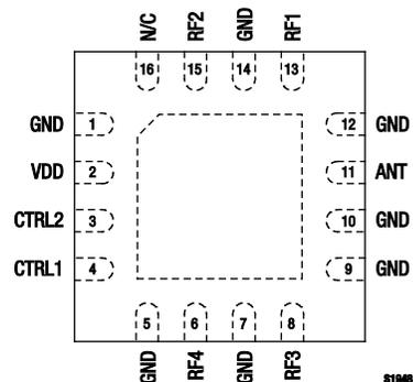
Figure 2. SKY13380-350LF Pinout – 16-Pin QFN (Top View)
