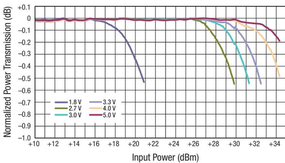
Figure 7. Compression vs Control Voltage (5.2 to 5.8 GHz)
