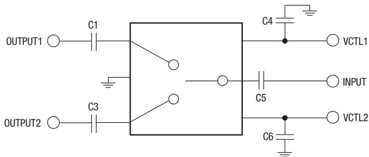
C1, C3, and C5 are DC blocking capacitors (100 pF)
