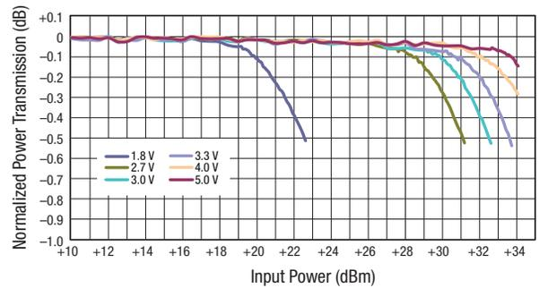
Figure 6. Compression vs Control Voltage (2450 MHz)
