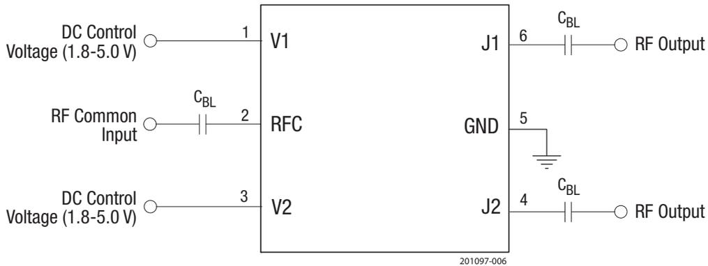
$C_{BL} = 47 \text{ pF}$  for >1 GHz operation.
