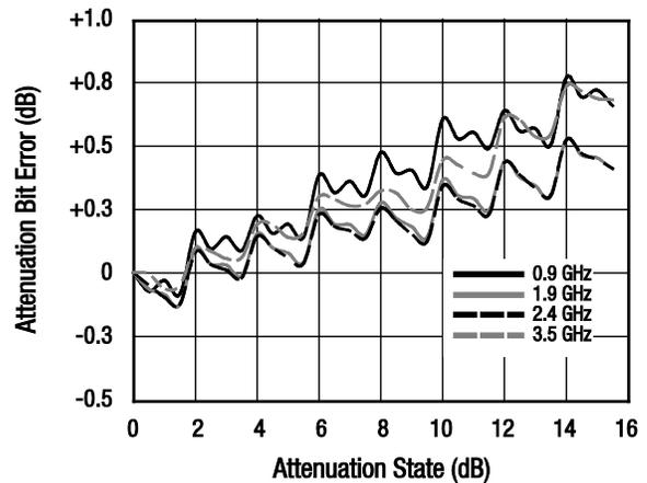
Figure 8. Attenuation Bit Error vs Attenuation State
