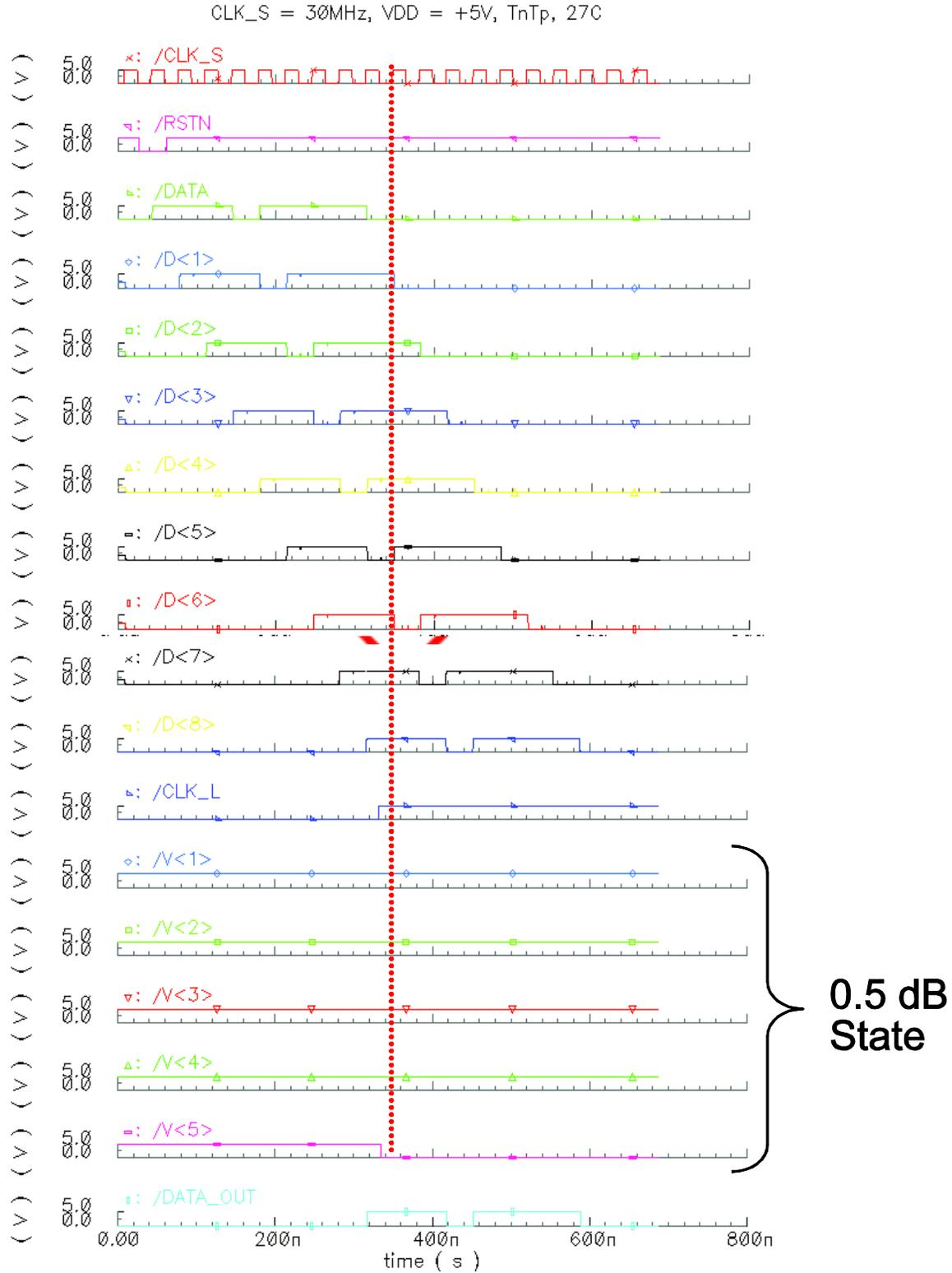
Figure 4. Example for Setting 0.5 dB State
