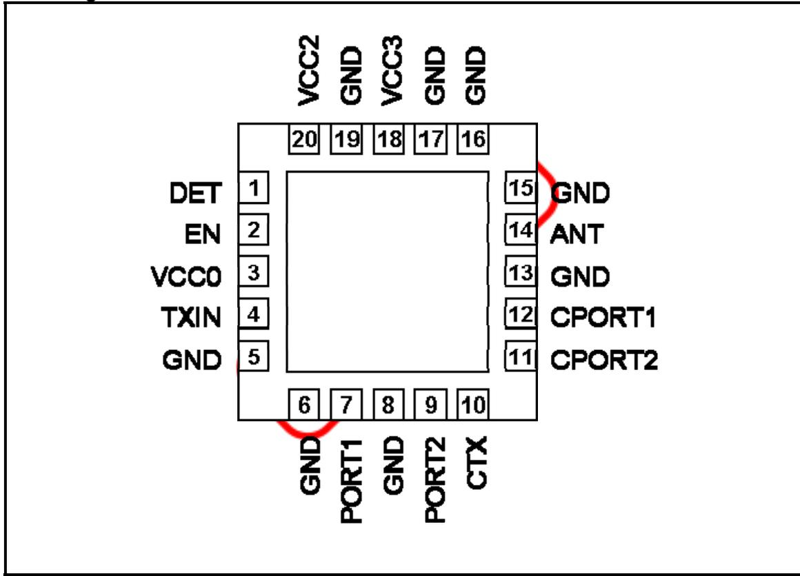
Figure 2: SE2614BT Pin Out (Top View Through Package)
