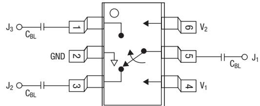
DC blocking capacitors (C<sub>BL</sub>) must be supplied externally for positive voltage operation. C<sub>BL</sub> = 100 pF for operation >500 MHz.
