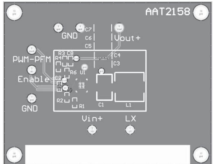
**Figure 4: AAT2158 Evaluation Board Bottom Side Layout.**
