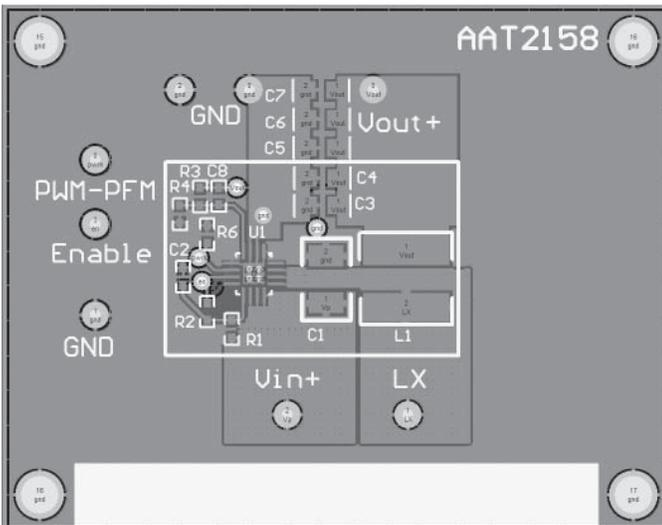
**Figure 3: AAT2158 Evaluation Board Top Side Layout.**
