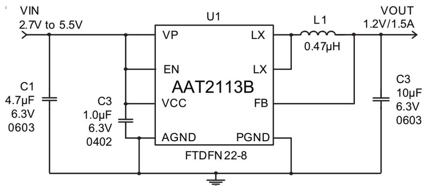
**AAT2113B****3.3MHz, Fast Transient 1.5A Step-Down Converter in an 2mm x 2mm Package****Pin Descriptions**
