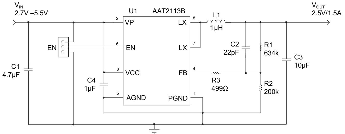
**Figure 8: AAT2113B Application Schematic for 2.5V Output Voltage.**
