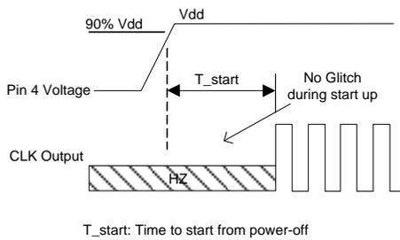
**Figure 4. Startup Timing (OE/ST Mode)**<sup>[9]</sup>
