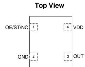
Figure 1. Pin Assignments
