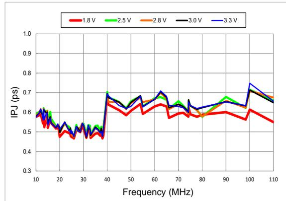
Figure 15. RMS Integrated Phase Jitter Random (900 kHz to 20 MHz) vs Frequency<sup>[11]</sup>
