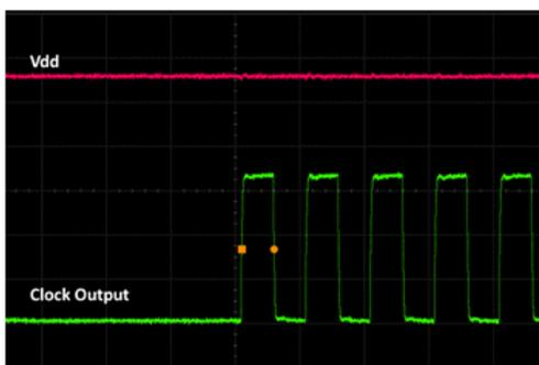
**Figure 18. Startup Waveform vs. Vdd
