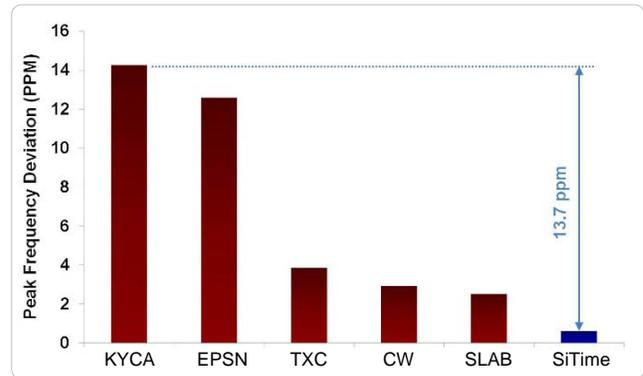
Figure 6. Shock Robustness<sup>[6]</sup>
