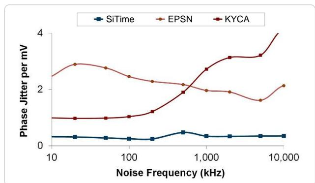
Figure 4. Power Supply Noise Rejection<sup>[4]</sup>
