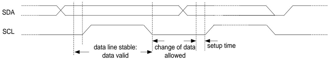
**Figure 42. Data and clock timing relation in I<sup>2</sup>C bus**
