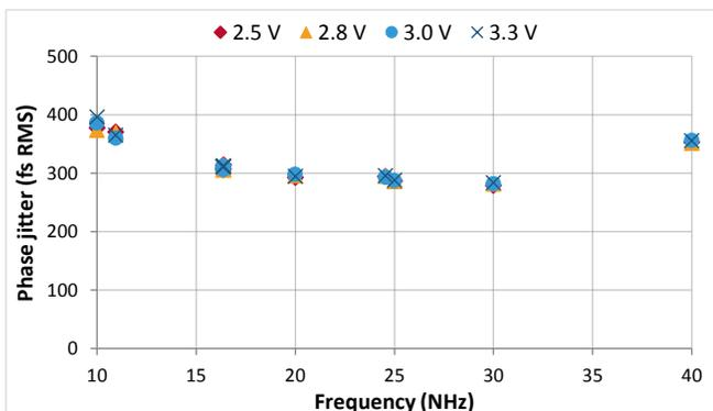
Figure 33. RMS Phase Jitter, VCTCXO (Clipped Sine)
