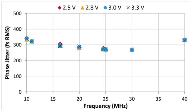
Figure 23. RMS Phase Jitter, TCXO & DCTCXO (LVCMOS)
