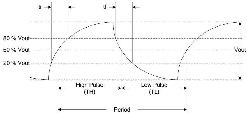
Figure 16. Clipped Sinewave Waveform Diagram<sup>[12]</sup>
