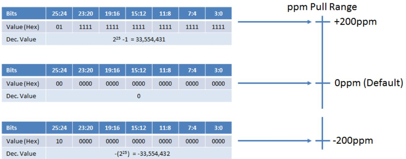
Figure 41. Pull Range and Frequency Control Word
