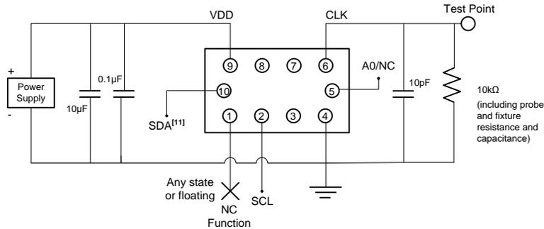
Figure 13. Clipped Sinewave Test Circuit (I<sup>2</sup>C Control), DCTCXO mode for AC and DC Measurements
