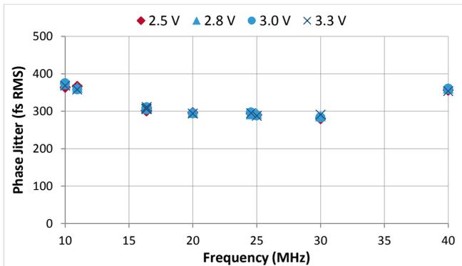
Figure 31. RMS Phase Jitter, TCXO & DCTCXO (Clip Sine)
