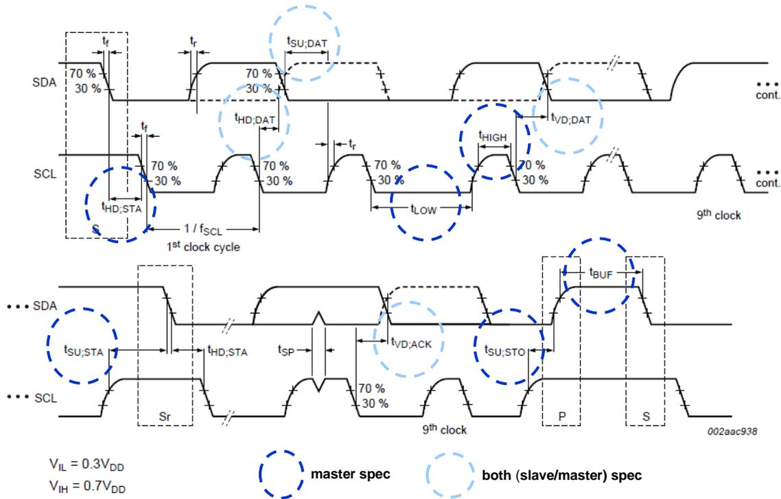
Figure 48. I<sup>2</sup>C Timing Diagram
