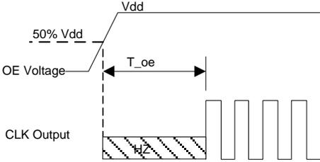
T\_oe: Time to re-enable the clock output
