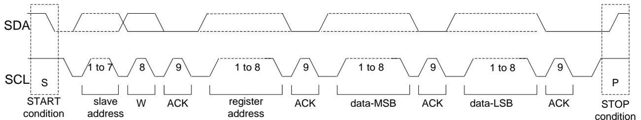
Figure 45. Parallel data byte format, write operation
