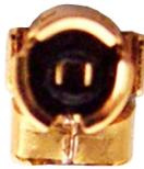
Female centre plug, mates by slotting around male. In most circumstances, antenna cables and cable assemblies are terminated with the U.FL/IPEX Male connector.
