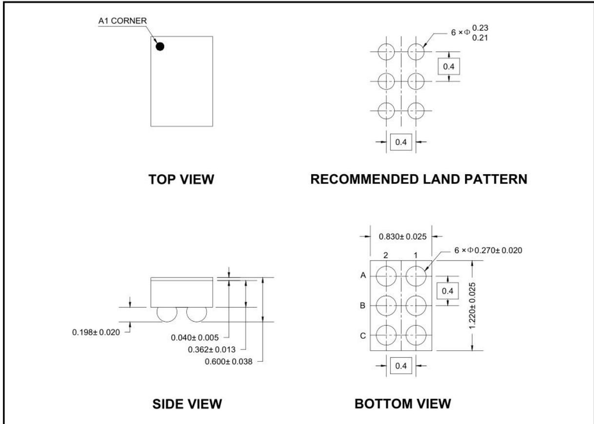
NOTE: All linear dimensions are in millimeters.
