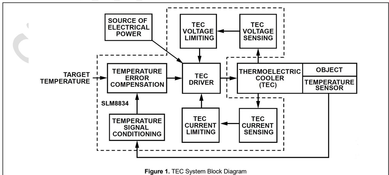
Figure 1. TEC System Block Diagram
