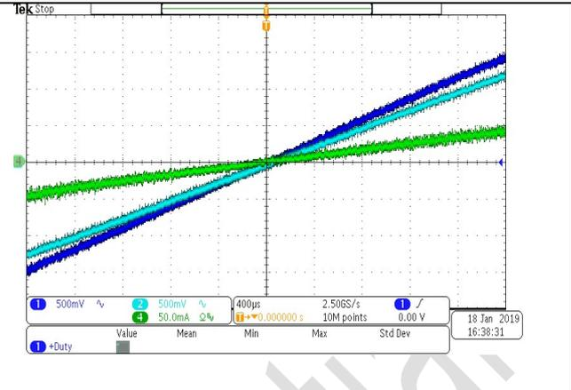
**Figure 11.** Zero Crossing TEC Current Zoom-in from Heating to Cooling (Line 1: LDR (TEC+), Line 2: SFB (TEC-), Line 4: ITEC)
