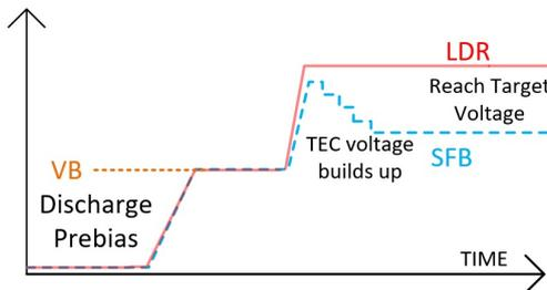
Figure 15. Soft Start Profile in Cooling Mode
