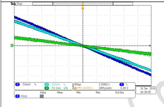
**Figure 12.** Zero Crossing TEC Current Zoom-in from Cooling to Heating (Line 1: LDR (TEC+), Line 2: SFB (TEC-), Line 4: ITEC)
